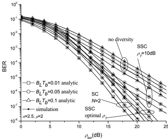
Fig. 2. Dependence of BER on average bit SNR for different values of parameter  $B_L T_b$  in the case of QPSK.
