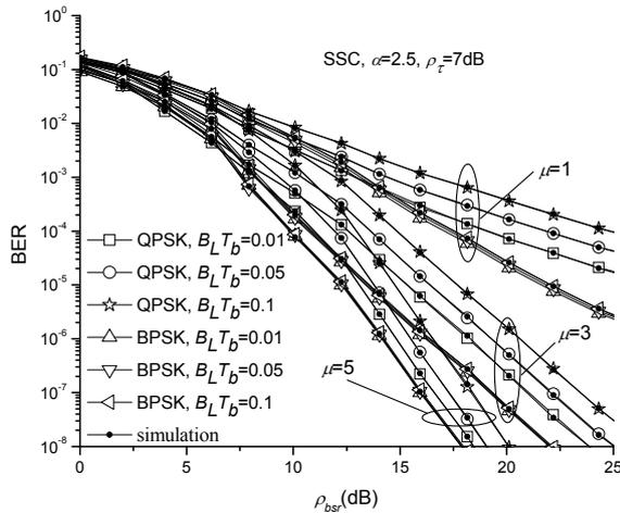
Fig. 4. Dependence of BER on the average bit SNR for different values of  $B_L T_b$  and fading parameter  $\mu$  in the case of QPSK and BPSK.
