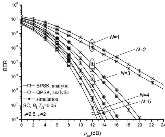
Fig. 5. Influence of diversity order on BPSK and QPSK signal detection.
