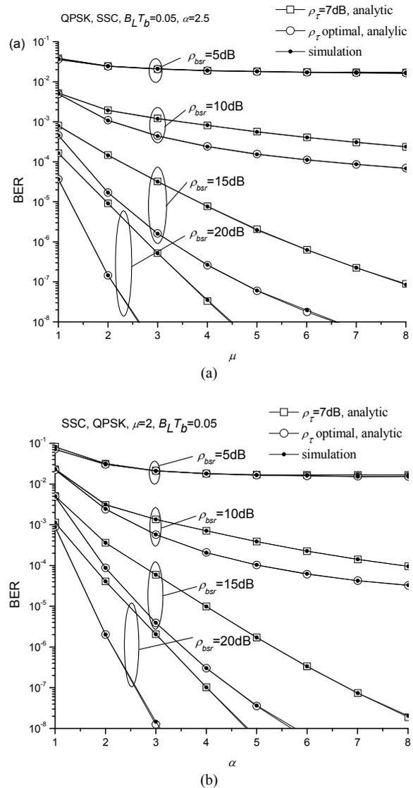
Fig. 3. Dependence of BER on the fading parameter  $\mu$  (a) and  $\alpha$  (b) for different values of the average bit SNR in case of QPSK.
