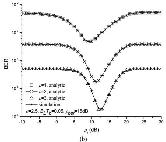
Fig. 1. (a) Dependence of BER on switching threshold for different values of average bit SNR in the case of QPSK. (b) Dependence of BER on switching threshold for different values of fading severity in the case of QPSK.
