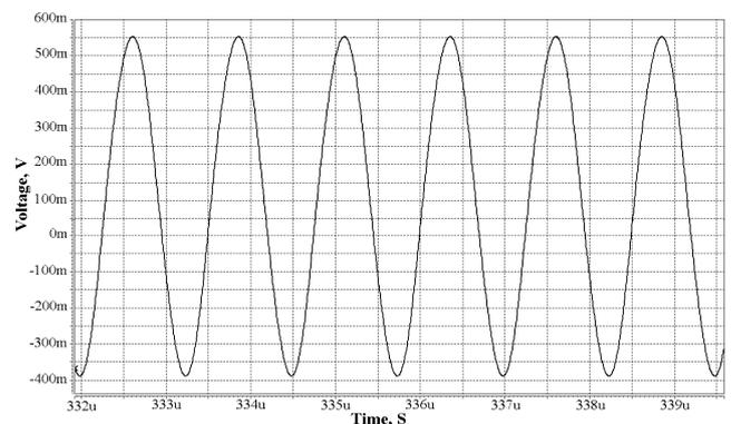
Fig. 9. Simulated output waveform of Fig. 2 with  $C_1 = 30$  pF,  $C_2 = 40$  pF,  $R_1 = 6$  k $\Omega$ ,  $R_2 = 5$  k $\Omega$  and  $R_3 = 10$  k $\Omega$ .
