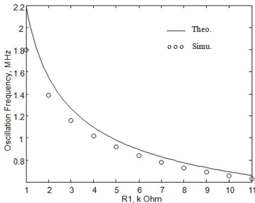
Fig. 6. Simulation results of the oscillation frequency of Fig. 1 by varying the value of the resistor  $R_1$ .
