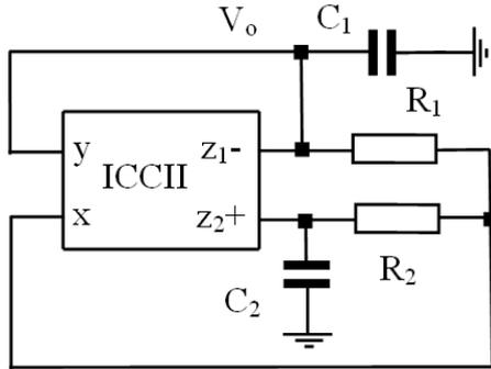
Fig. 1. The first proposed ICCII based sinusoidal oscillator.
