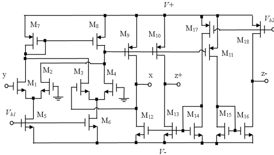
Fig. 4. CMOS realization of the ICCII [22].
