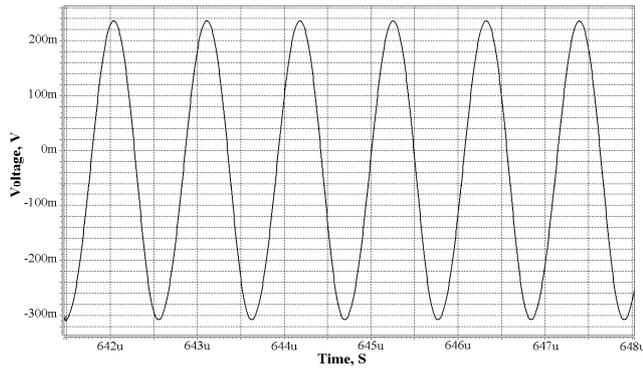
Fig. 5. Simulated output waveform of Fig. 1 with  $C_1 = 15$  pF,  $C_2 = 35$  pF,  $R_1 = 5$  k $\Omega$ ,  $R_2 = 20$  k $\Omega$ .
