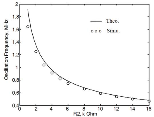
Fig. 8. Simulation results of the oscillation frequency of Fig. 1 by varying the value of the resistor  $R_2$ .
