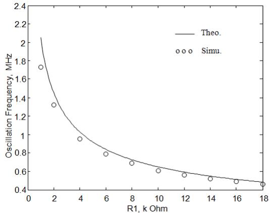
Fig. 10. Simulation results of the oscillation frequency of Fig. 2 by varying the value of the resistor R<sub>1</sub>.
