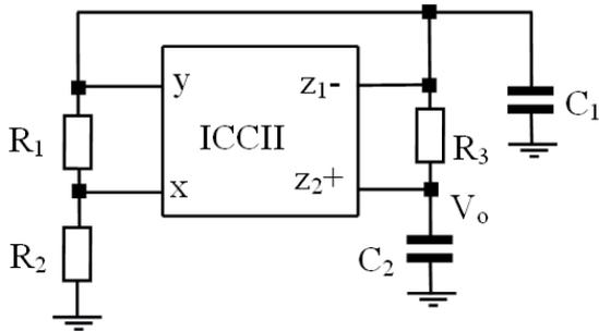
Fig. 2. The second proposed ICCII based sinusoidal oscillator.
