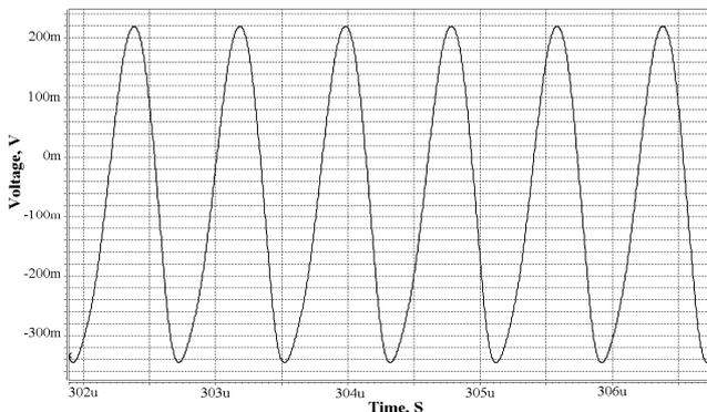
Fig. 7. Simulated output waveform of Fig. 1 with  $C_1 = 25$  pF,  $C_2 = 55$  pF,  $R_1 = 10$  k $\Omega$ ,  $R_2 = 5$  k $\Omega$ .
