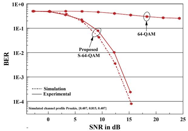
Fig. 15. BER performances of CMA blind equalizer for experimental and simulated channels in 64-QAM and S-64-QAM modulations.
