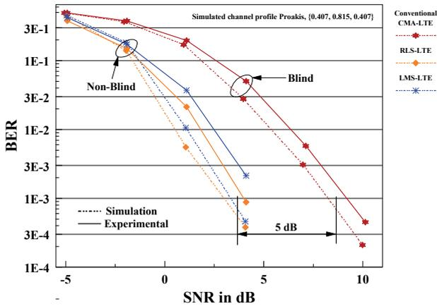
Fig. 13. Comparative BER performances of non-blind and blind equalizers for experimental and simulated channels in S-16-QAM modulation.
