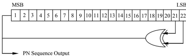
Fig. 3. Spreading PN sequence generator.
