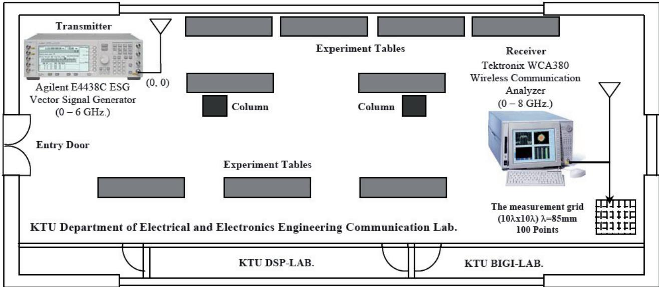
Fig. 8. The test area and measurement grid with 100 points.
