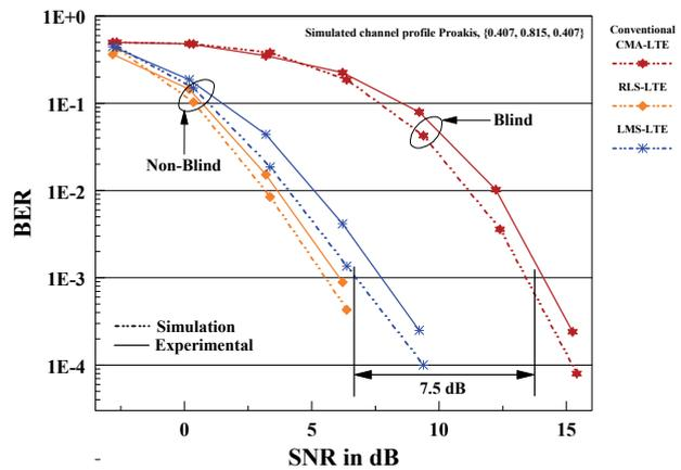
Fig. 16. Comparative BER performances of non-blind and blind equalizers for experimental and simulated channels in S-64-QAM modulation.
