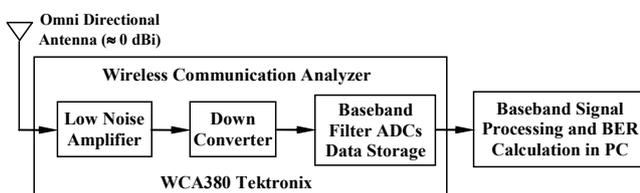
Fig. 7. Receiver of experimental radio set.
