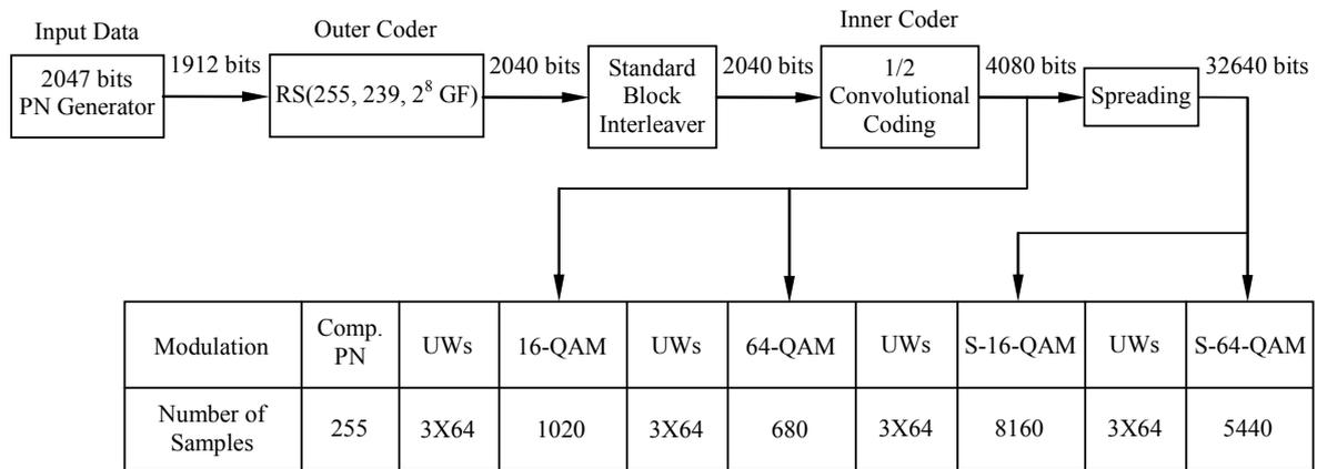
Fig. 6. Transmit data packet structure.
