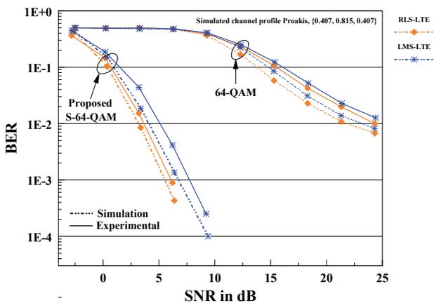
Fig. 14. BER performances of non-blind equalizers for experimental and simulated channels in 64-QAM and S-64-QAM modulations.
