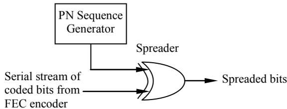
Fig. 2. The spreading process.
