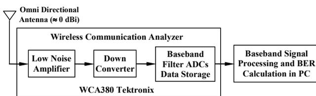
Fig. 7. Receiver of experimental radio set.
