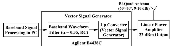
Fig. 5. Transmitter of Experimental Radio Set.
