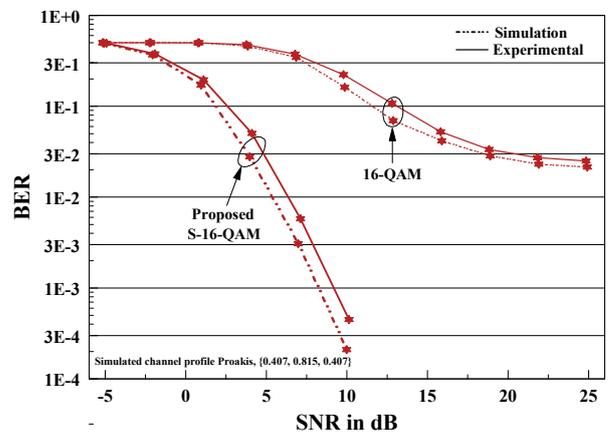
Fig. 12. BER performances of CMA blind equalizer for experimental and simulated channels using 16-QAM and S-16-QAM modulations.
