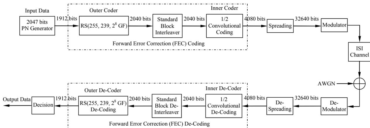
Fig. 1. The WiMAX model in single carrier wireless communication systems.
