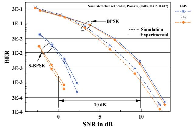
Fig. 4. BER performances of non-blind equalizers for experimental and simulated channels using BPSK and S-BPSK modulations.
