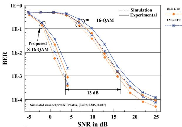
Fig. 11. BER performances of non-blind equalizers for experimental and simulated channels using 16-QAM and S-16-QAM modulations.
