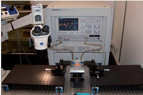
Fig. 5. Photograph of the test setup for the experimental validation of CBCPW on BCB substrate.
