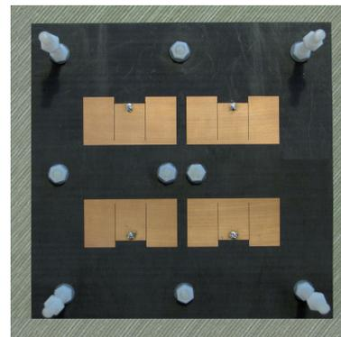
Fig. 15. Photograph of the fabricated array with E-shaped patches and washer (the radome was removed).
