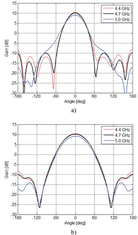
Fig. 6. Radiation patterns of the stacked-patch antenna: E-field (a), H-field (b).
