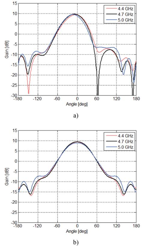
Fig. 12. Radiation patterns of the U-slot patch antenna: E-field (a), H-field (b).
