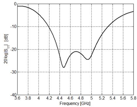
**Fig. 2.** Reflection coefficient of the aperture-fed antenna.
