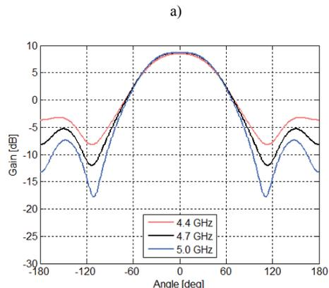
**Fig. 3.** Radiation patterns of the aperture-fed antenna: E-field (a), H-field (b).
