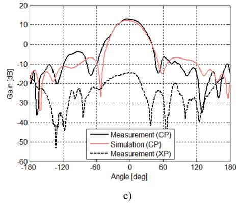
**Fig. 23.** Radiation patterns (E-field) of the array with U-slot patches: 4.4 GHz (a), 4.7 GHz (b), 5.0 GHz (c).
