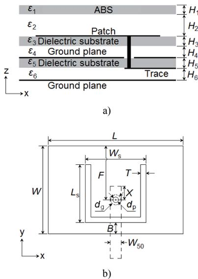
Fig. 19. Schematics of the U-slot patch antenna with ABS: side view (a), top view (b).
