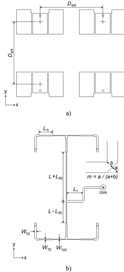
Fig. 14. Schematics of the array with E-shaped patches and washer: top view (a), feeding network (b).
