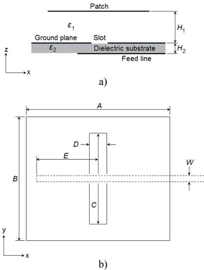
**Fig. 1.** Schematics of the aperture-fed antenna: side view (a), top view (b).
