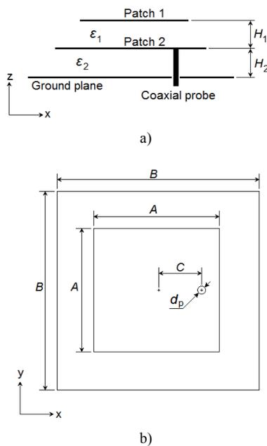
Fig. 4. Schematics of the stacked-patch antenna: side view (a), top view (b).
