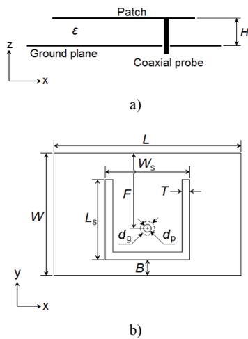
Fig. 10. Schematics of the U-slot patch antenna: side view (a), top view (b).
