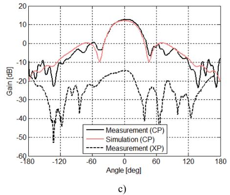
**Fig. 24.** Radiation patterns (H-field) of the array with U-slot patches: 4.4 GHz (a), 4.7 GHz (b), 5.0 GHz (c).
