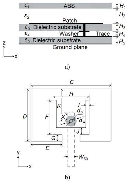
Fig. 13. Schematics of the E-shaped patch antenna with washer and ABS: side view (a), top view (b).
