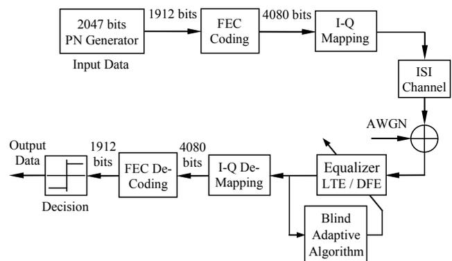
Fig. 2. The block scheme of the IEEE 802.16-2004 SC radio physical layer.
