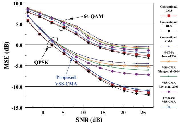
Fig. 8. Comparison of the MSE versus SNR performances of the blind and non-blind equalizers for QPSK and 64-QAM.
