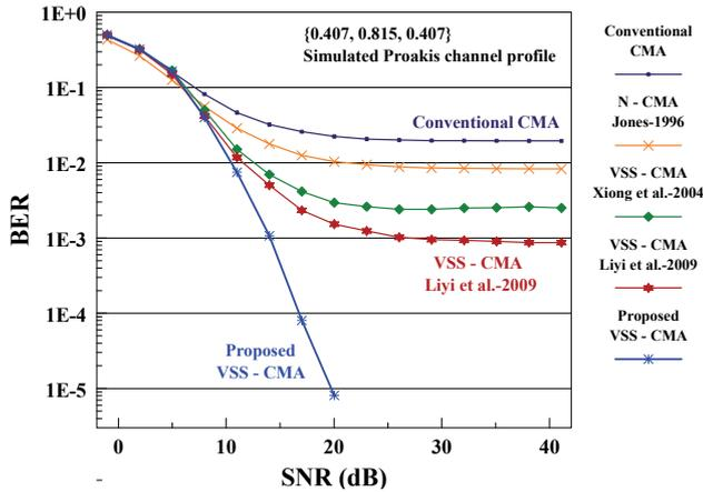
Fig. 4. Comparison of the coded BER performances of the blind adaptive channel equalizers.
