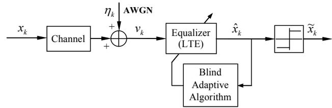
Fig. 1. The system model of adaptive blind equalization system.
