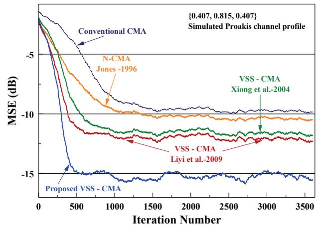
Fig. 3. Comparison of the MSE performances of the blind adaptive channel equalizers.
