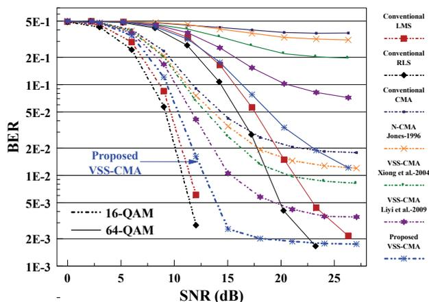
Fig. 10. Comparison of the coded BER versus SNR performances of the blind and non-blind equalizers for 16-QAM and 64-QAM.
