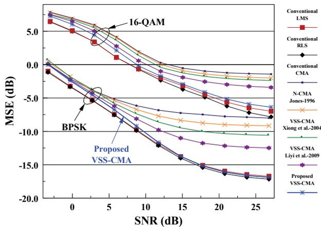
Fig. 7. Comparison of the MSE versus SNR performances of the blind and non-blind equalizers for BPSK and 16-QAM.
