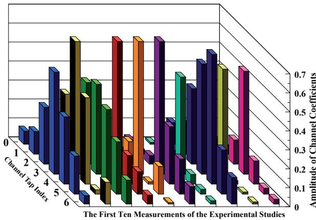
Fig. 6. A sampled channel profile obtained from the experimental IEEE 802.16-2004 SC radio set.
