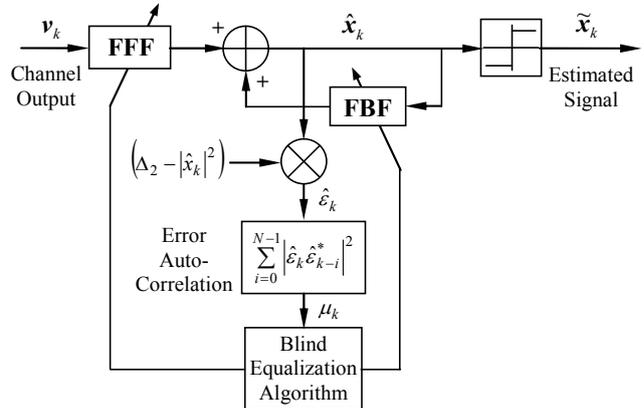
Fig. 5. The proposed variable step size CMA algorithm based on error autocorrelation with SDFE.
