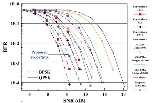
Fig. 9. Comparison of the coded BER versus SNR performances of the blind and non-blind equalizers for BPSK and QPSK.
