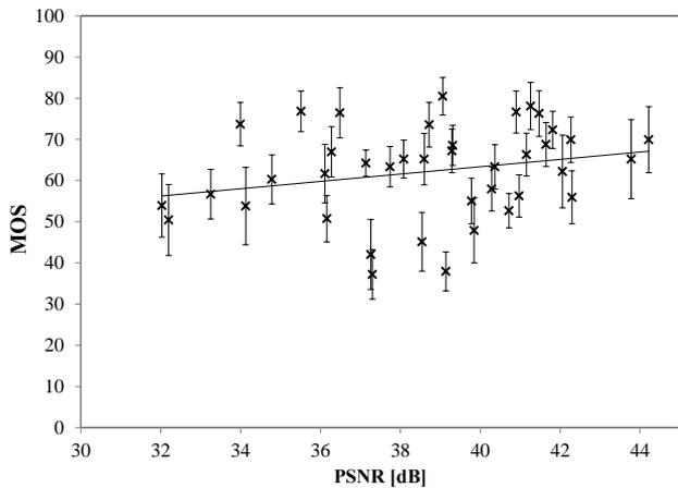
**Fig. 6.** Scatter plot graph showing the dependency between sequence PSNR and average user score (DMOS) captured at the end of continuous evaluation.
