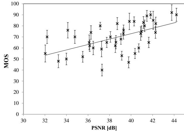
**Fig. 8.** Scatter plot graph showing the dependency between sequence PSNR and mean opinion score recorded in a gray-image interval after each sequence.
