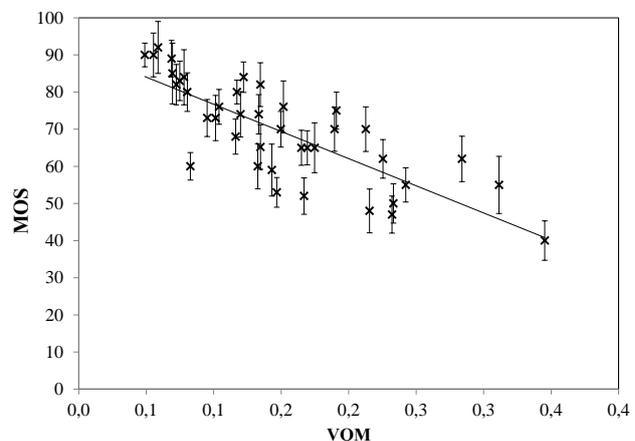
**Fig. 9.** Scatter plot graph showing the dependency between sequence VQM and mean opinion score recorded in a gray-image interval after each sequence.
