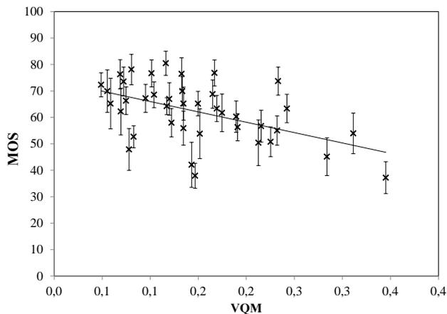
**Fig. 7.** Scatter plot graph showing the dependency between sequence VQM and mean opinion score captured at the end of continuous evaluation.
