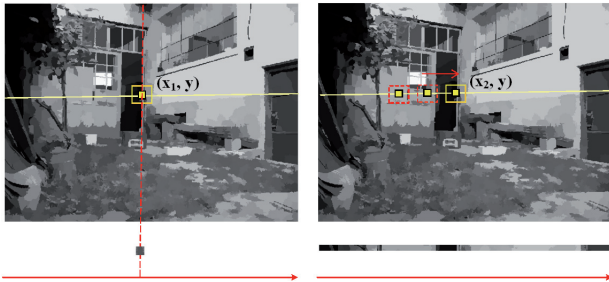
Fig. 10. Correspondence using window – based matching (rectified images).
