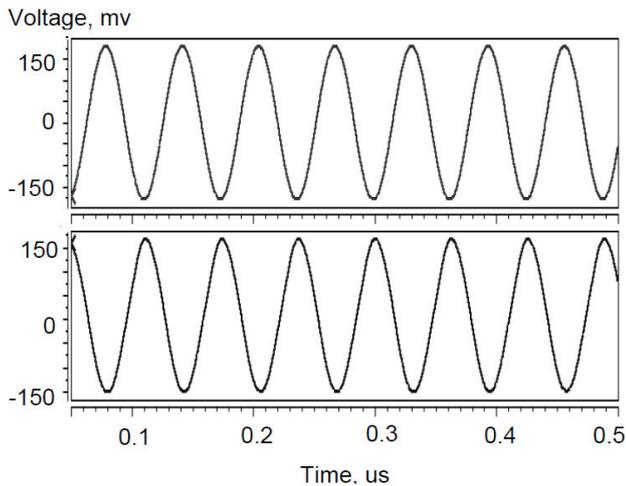
Fig. 6. Time-domain input (upper signal) and output signal waveforms to demonstrate the ac dynamic range of the proposed filter.
