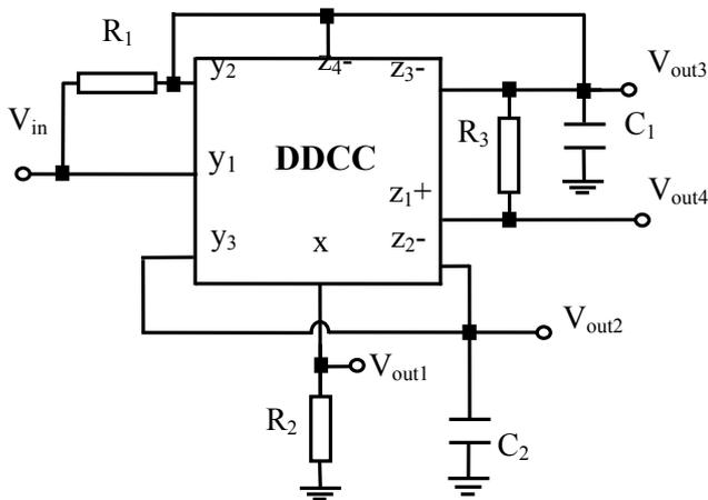
**Fig. 1.** The proposed voltage-mode highpass, bandpass, lowpass and notch biquadratic filter using single DDCC.
