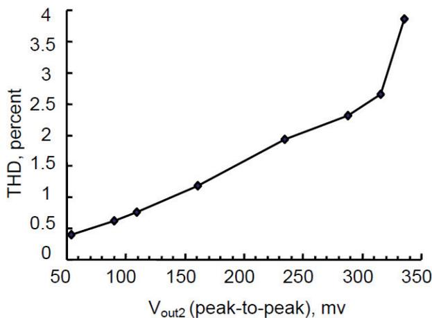
Fig. 7. THD analysis results of the proposed bandpass filter.
