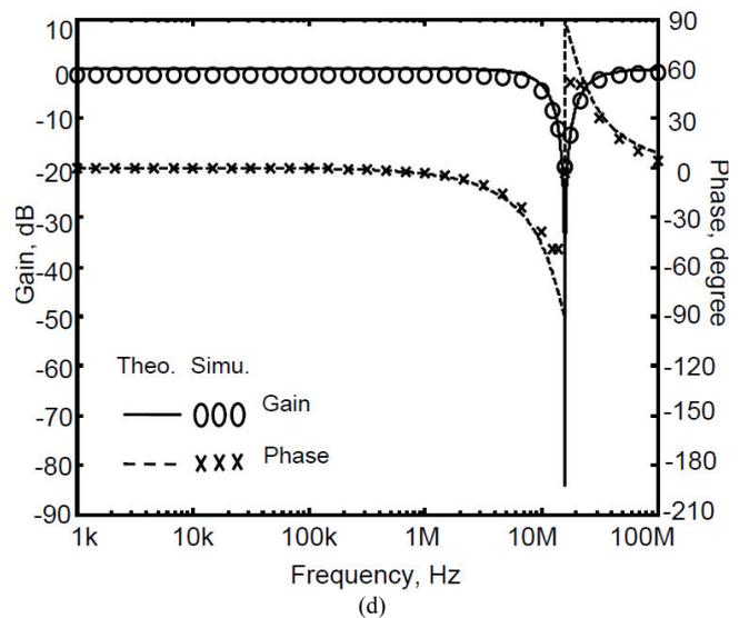
Fig. 4. Simulated frequency responses: (a) for the highpass filter ( $V_{out1}$ ) of Fig. 1, (b) for the bandpass filter ( $V_{out2}$ ) of Fig. 1, (c) for the lowpass filter ( $V_{out3}$ ) of Fig. 1, (d) for the notch filter ( $V_{out4}$ ) of Fig. 1.
