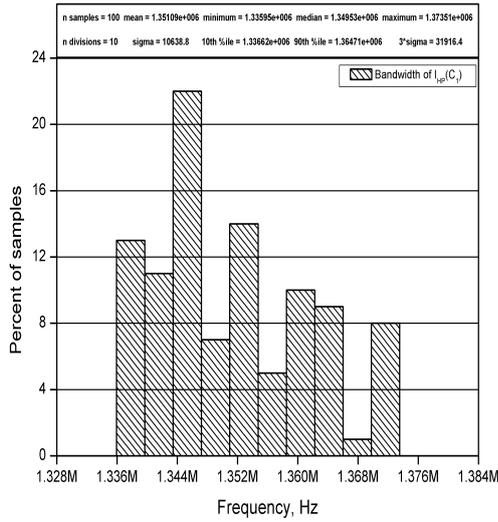
Fig. 9. MC analysis for the first proposed filter.
