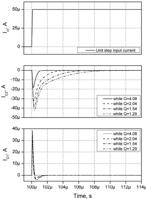
Fig. 14. The responses to the input unit step signal of the second universal filter.
