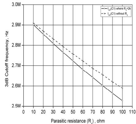
Fig. 8. Effects of the resistor  $R_3$  on the proposed CM universal filters.
