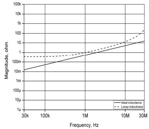
Fig. 7. AC analysis results for the lossy inductor.
