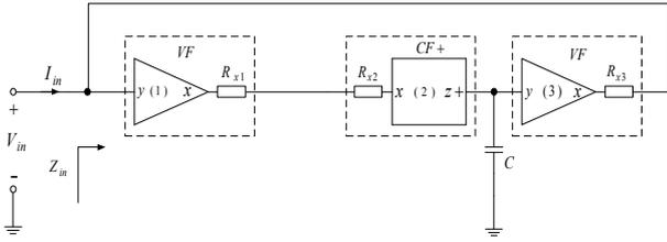
Fig. 3. Proposed active inductor circuit.
