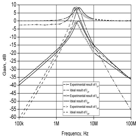
Fig. 19. Experimental results of the first suggested CM second-order universal filter.
