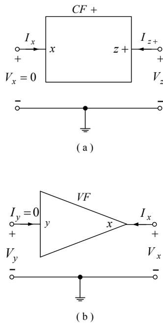
Fig. 1. Symbolic representation of (a) CF+, (b) VF.
