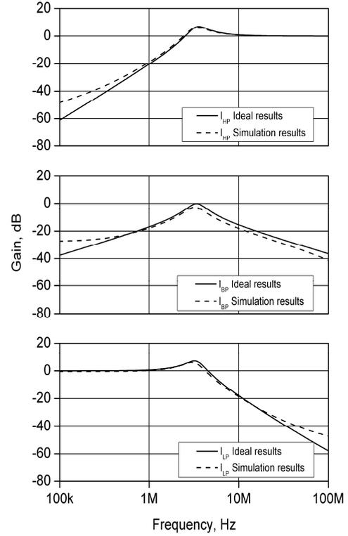
Fig. 12. The first proposed filter TFs in AC analysis.
