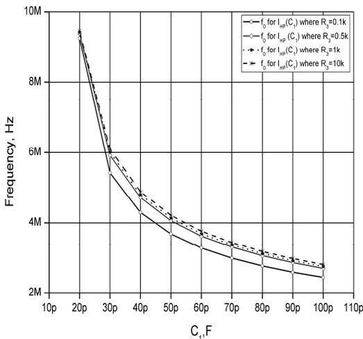
Fig. 11. Impact on the 3dB cutoff frequency of  $I_{C1}$  by changing  $C_1$  and  $R_3$ .
