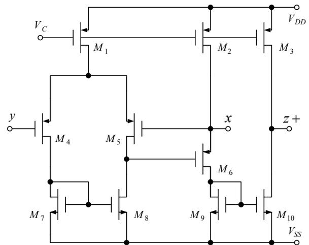
Fig. 2. CMOS CCII internal structure of [16].
