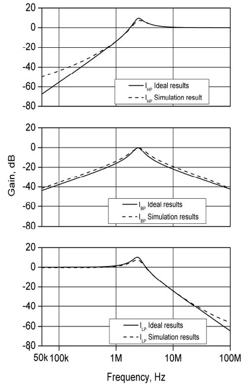
Fig. 13. AC analysis results for the reorganized filter.
