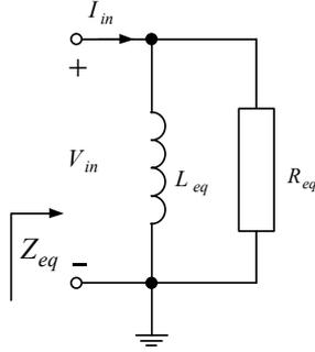
Fig. 4. Symbolic equivalent circuit of the proposed inductor.
