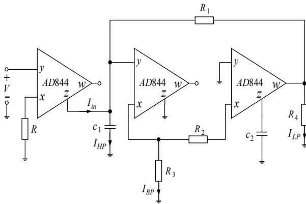
Fig. 18. Test circuit designed with AD844 ICs.
