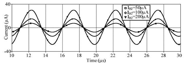
Fig. 7. Output currents for different values of  $I_{B2}$ .
