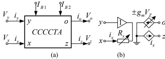
Fig. 1. CCCCTA: (a) Symbol, (b) Equivalent circuit.
