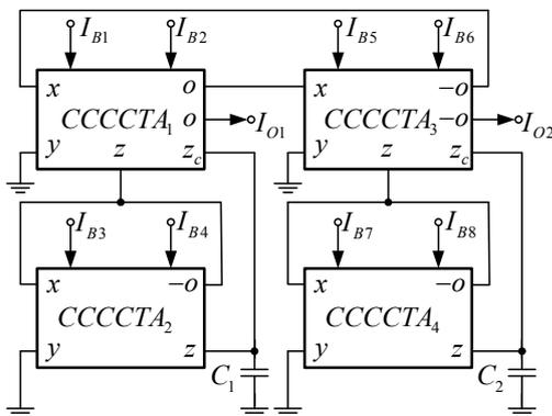
Fig. 9. Current-mode quadrature oscillator.
