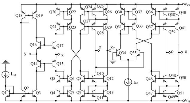
Fig. 2. Schematic of the BJT CCCCTA.
