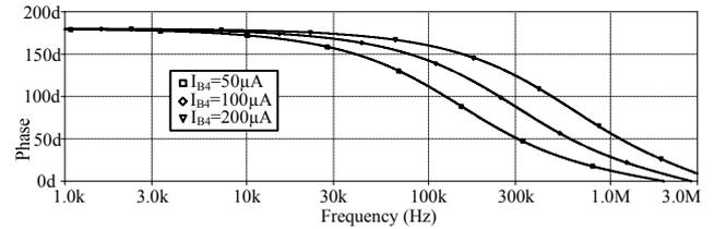
Fig. 5. Simulated phase responses of the proposed allpass filter when  $I_{B4}$  is varied.
