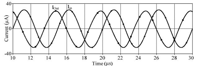
Fig. 6. Filter response to a 0.2 MHz sinusoidal input signal.
