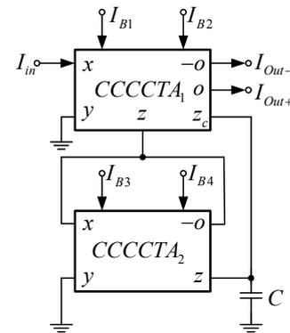
Fig. 3. Proposed gain controllable APF.
