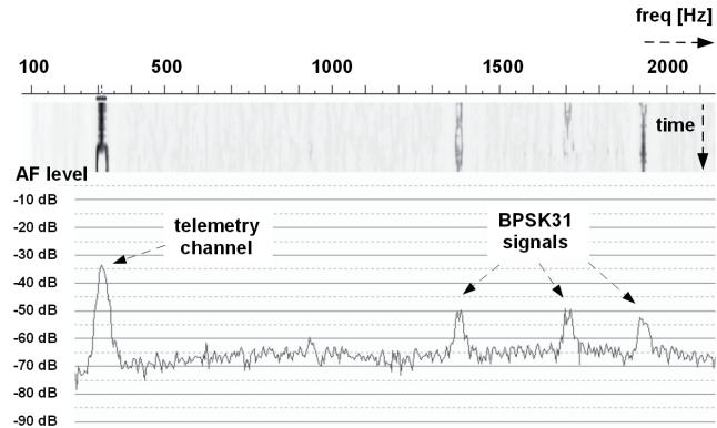
Fig. 14. Base-band spectrum (and spectrum in time) of de-modulated signal from 0 to 2000 Hz.
