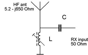
Fig. 9. HF antenna matching circuit (L = 2.8 uH, C = 2.7 pF).
