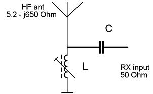
Fig. 9. HF antenna matching circuit ( $L = 2.8\ \mu H$ ,  $C = 2.7\ pF$ ).
