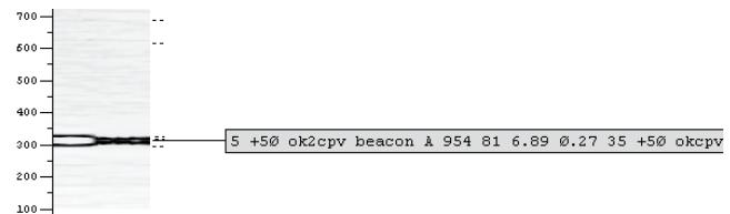
Fig. 15. Spectrum in time and decoded data of the telemetry channel. (Horizontal axis - time, vertical axis - frequency in Hz).
