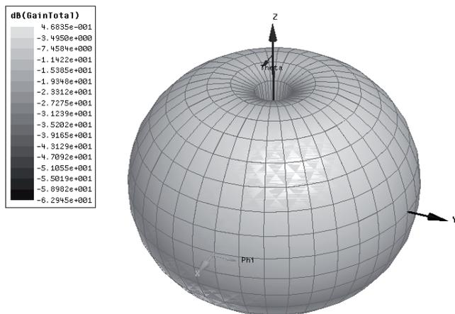
Fig. 13. Expected radiation pattern of the receiver antenna. Antenna is oriented in z-axis.
