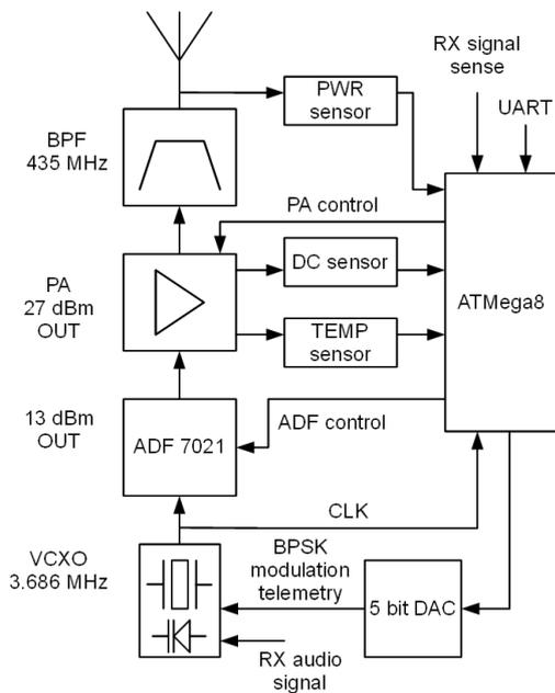
Fig. 2. Transmitter block diagram.
