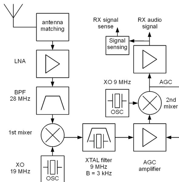
Fig. 1. Receiver block diagram.
