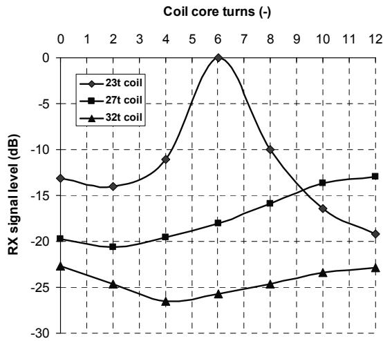
Fig. 12. Tuning the matching circuit of the RX antenna. RX signal level is normalized to the best result.
