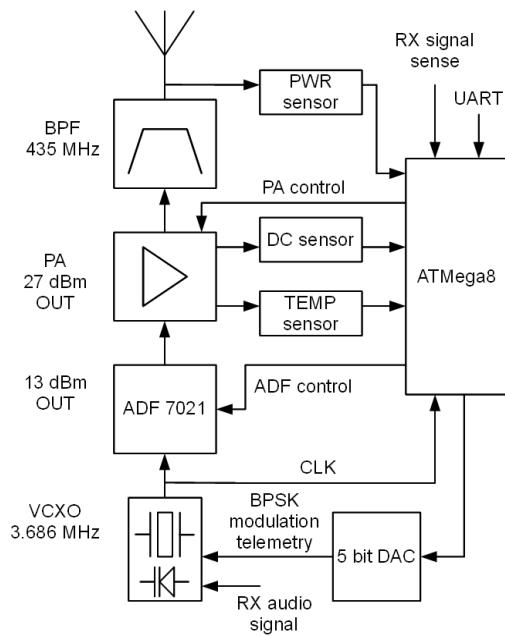
Fig. 2. Transmitter block diagram.
