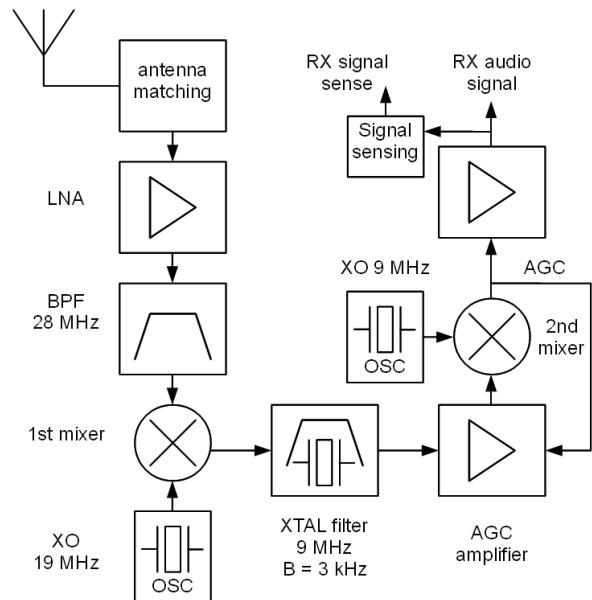
Fig. 1. Receiver block diagram.
