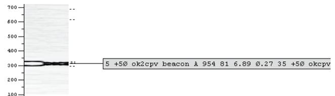
Fig. 15. Spectrum in time and decoded data of the telemetry channel. (Horizontal axis - time, vertical axis - frequency in Hz).
