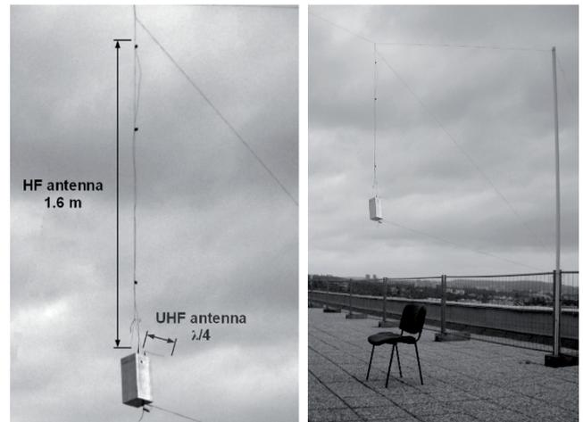
Fig. 10. Tests of HF antenna with a model of a double Cube-Sat.
