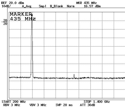
Fig. 5. Wideband output spectrum of the transmitter (with 10 dB attenuator).
