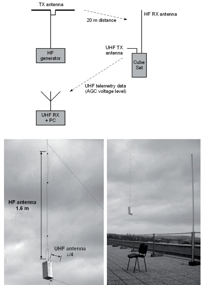
Fig. 10. Tests of HF antenna with a model of a double Cube-Sat.
