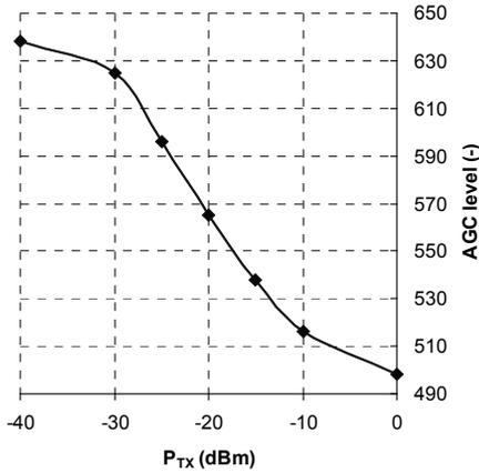
Fig. 11. AGC level after A/D conversion vs. generator output power.
