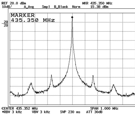
Fig. 6. Output spectrum of the transmitter in 1 MHz bandwidth (with 10 dB attenuator).
