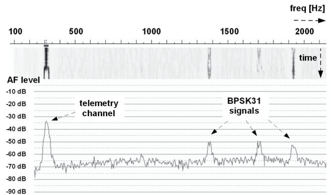
Fig. 14. Base-band spectrum (and spectrum in time) of demodulated signal from 0 to 2000 Hz.
