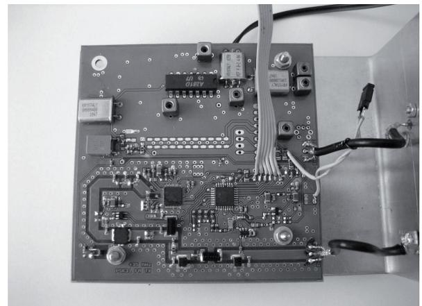
Fig. 4. The prototype board attached to a test-bed with connected programming cable.
