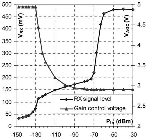
Fig. 8. Output signal amplitude and AGC voltage vs. input signal.
