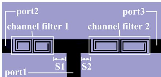
Fig. 7. Configuration of the proposed diplexer.
