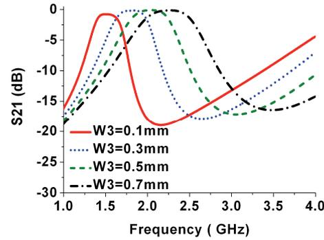
Fig. 5. Simulated S21 for ASSRs with different W3. In this case, L1 = 5.5 mm and W4 = 0.2 mm.
