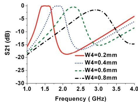
Fig. 6. Simulated S21 for ASSRs with different W4. In this case, L1 = 5.5 mm and W3 = 0.1 mm.
