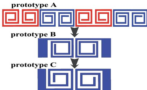
Fig. 1. Schematic representation of the improvement of spiral-based resonators.
