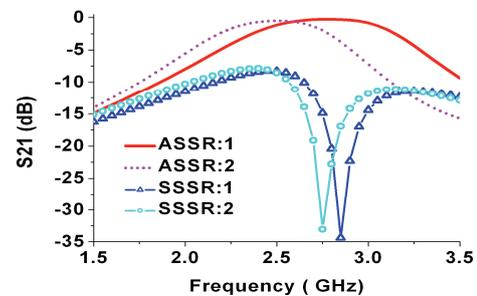
Fig. 3. Comparison of S21 of ASSR and SSSR. In this figure, ‘1’ represents the combination of the geometrical parameters: L1 = 4.8 mm, W3 = 0.7 mm, W4 = 0.2 mm. ‘2’ represents the combination: L1 = 5.4 mm, W3 = 0.7 mm, W4 = 0.2 mm.
