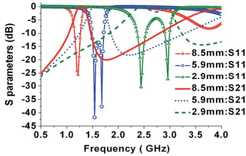
Fig. 4. Simulated S-parameters for ASSRs with different L1. In this case, W3 = 0.1 mm and W4 = 0.3 mm.
