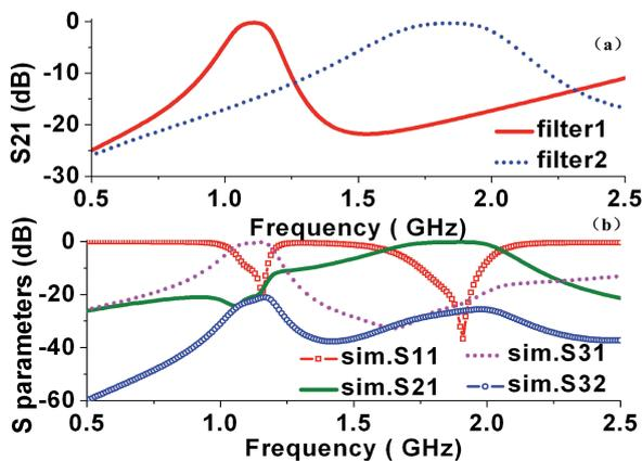
Fig. 8. (a) Simulated S21 for independently designed filter1 and filter2. (b) Simulated S-parameters for the proposed diplexer.
