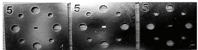
Fig. 1. Sample specimens prepared for empty, Teflon and unknown polymer using WR-05 waveguide steel holders.
