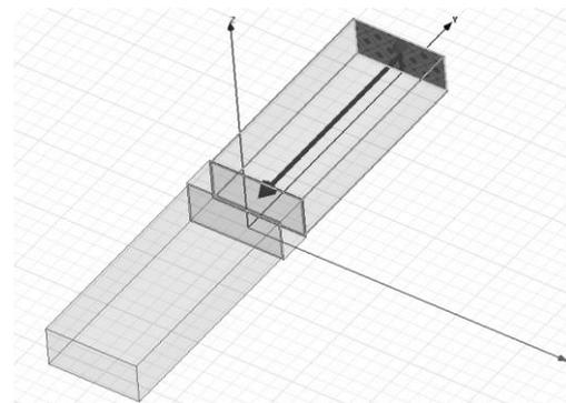
Fig. 3. Simulation structure in HFSS with de-embedded wave-port excitation.
