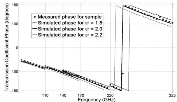
Fig. 8. Transmission coefficient phase for Teflon with  $\pm 10$  percent change in dielectric constant.
