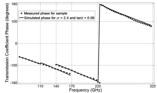
Fig. 7. Measured and simulated transmission coefficient phase for unknown polymer.
