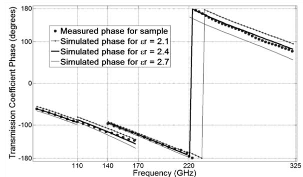
Fig. 9. Transmission coefficient phase for unknown polymer with  $\pm 12.5$  percent change in dielectric constant.
