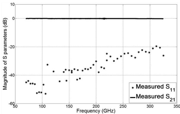
Fig. 5. Empty holder measurement in the frequency range of 75-325 GHz.
