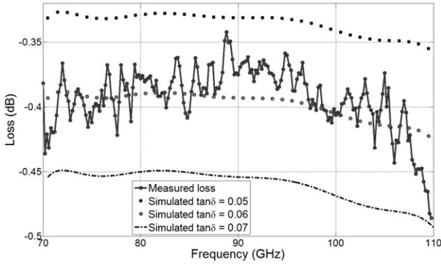
Fig. 10. Measured loss for unknown polymer compared with the simulated losses for different values of loss tangent.
