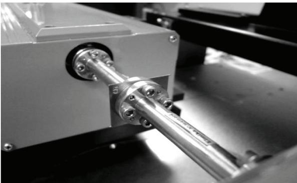
Fig. 2. WR-05 sample specimen placed in between the waveguide test heads.
