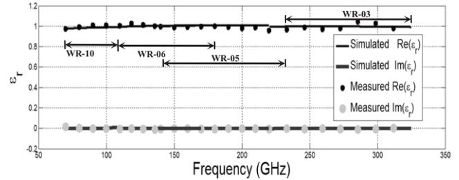
Fig. 11. Calculated dielectric constant for air (empty holder) using MNRW extraction technique.
