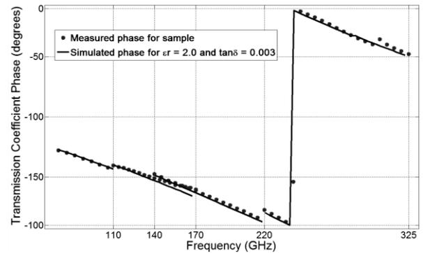
Fig. 6. Measured and simulated transmission coefficient phase for Teflon.
