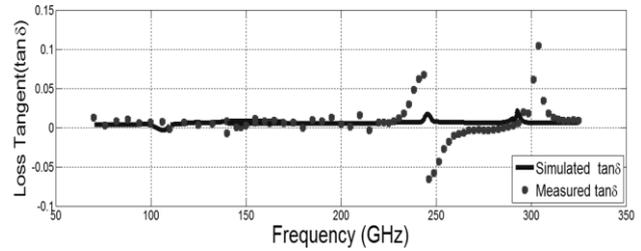
Fig. 12. Calculated dielectric constant and loss tangent for Teflon using MNRW extraction technique.
