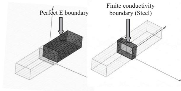
Fig. 4. Boundary condition assignment for the waveguide sections and the sample holder.
