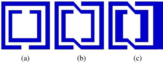
**Fig. 1.** Topologies for the rectangular SRR (a), conventional rectangular NB-SRR (b), and the proposed modified NB-SRR (c).
