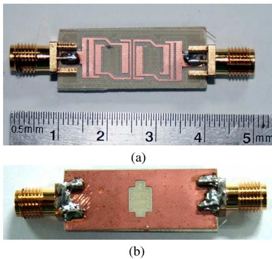
Fig. 7. Photograph of the proposed wideband bandpass filter (a) top view, (b) bottom view  $L_1 = 2.47$ ,  $L_2 = 1.17$ ,  $L_3 = 1.43$ ,  $L_4 = 0.78$ ,  $L_5 = 2.34$ ,  $L_6 = 2.27$ ,  $L_7 = 5.0$ ,  $W_1 = 7.54$ ,  $W_2 = 1.08$ ,  $W_2 = 1.3$ ,  $W_3 = 1.43$ ,  $W_4 = 0.52$ ,  $W_5 = 1.3$ ,  $W_6 = 4.7$ ,  $h_1 = 2.76$ ,  $h_2 = 0.845$ ,  $h_3 = 5.72$ ,  $h_4 = 1.04$  and  $g_1 = 0.39$  (unit: mm).
