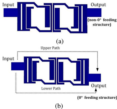
Fig. 5. (a) Non zero-degree feed structure and (b) zero-degree feed structure and the paths of the zero feed structure.
