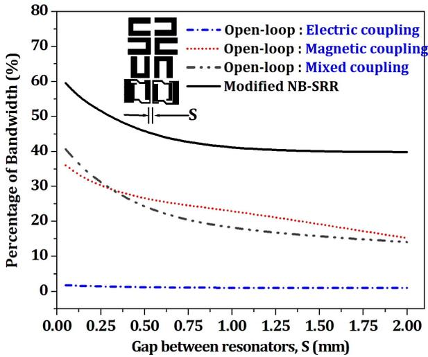
Fig. 3. Variation of percentage bandwidth with three couplings of conventional open loop resonator and the modified NB-SRR. (All of configurations used the same substrate.)
