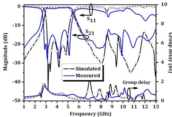
Fig. 8. Simulated and measured S-parameter and group delay results of the proposed wideband bandpass filter.
