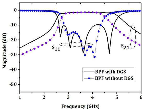
Fig. 4. Comparison of simulated S-parameter results for the wideband bandpass filter with and without the DGS.
