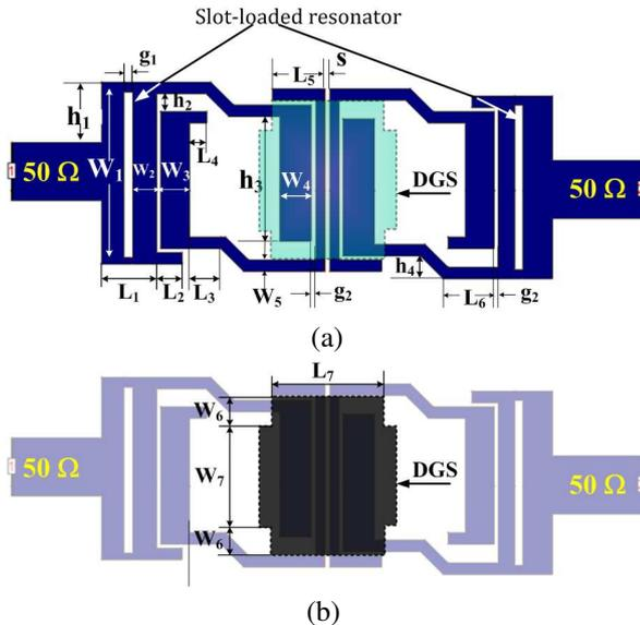
**Fig. 2.** The proposed wideband bandpass filter with wide stopband using metamaterial-based resonator (MBR), NB-SRRs and defected ground structure (DGS)(a) Top view and (b) Bottom view.
