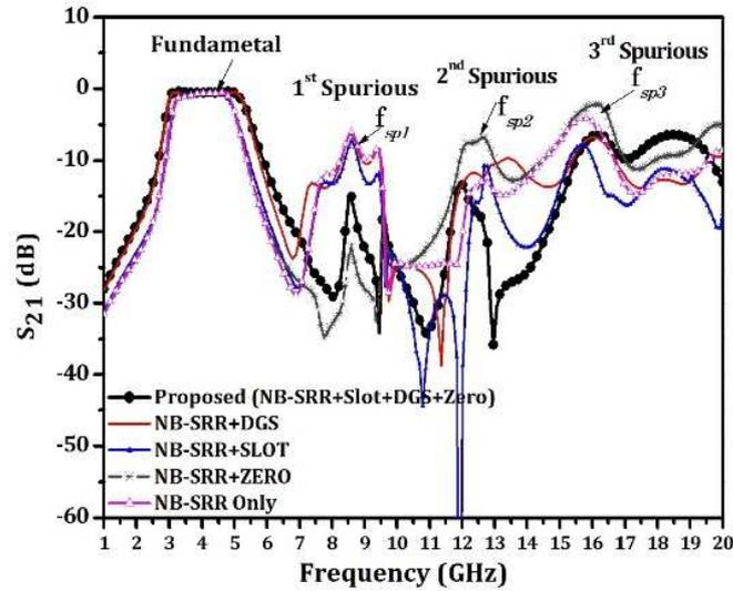
Fig. 6. Comparison of frequency responses ( $S_{21}$ ) of five wideband bandpass filter configurations.
