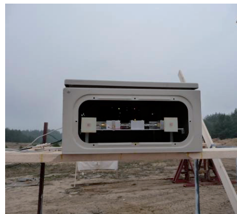
Fig. 1. Test CW radar sensor during practical tests at army shooting range.
