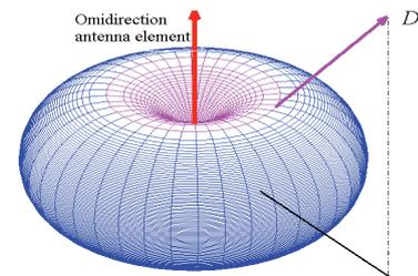
Fig. 3. Omnidirectional antenna radiation pattern.
