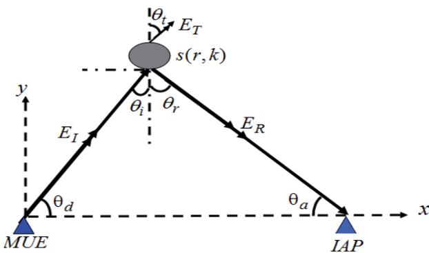
Fig. 4. Illustration of reflected and transmitted waves for wave incident upon a scatterer at oblique angle ( $E_R$  and  $E_T$  are the reflected and transmitted waves, respectively).
