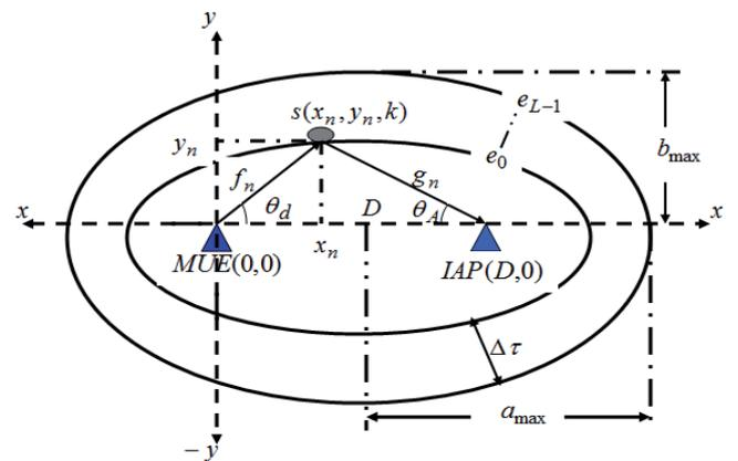
Fig. 2. Elliptical model for the UWB Infostation channel.
