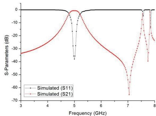
Fig. 5. Simulated S-Parameter responses of the CISIR.
