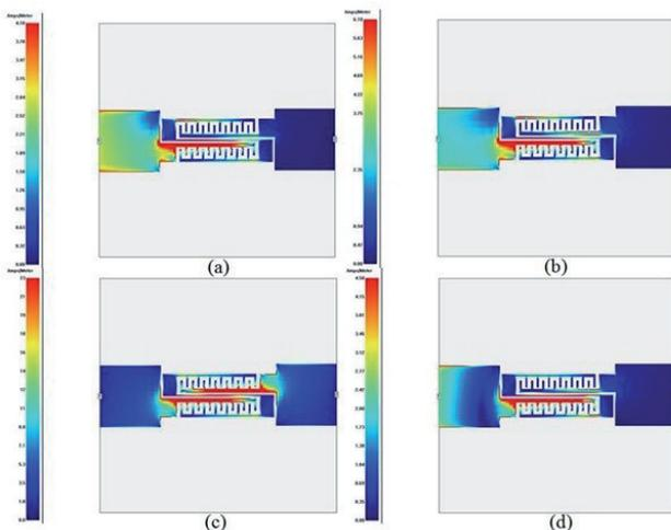
Fig. 4. The current distributions in the CISIR bandpass filter at (a) 3.5 GHz, (b) 4.0 GHz, (c) 5.0 GHz, (d) 6.0 GHz.
