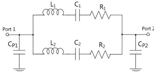
Fig. 3. Equivalent circuit of the CISIR bandpass filter.
