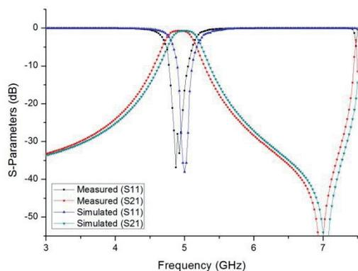
Fig. 7. Simulated and measured S-Parameter responses of the CISIR.
