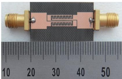
Fig. 6. Photograph of the fabricated CISIR bandpass filter.
