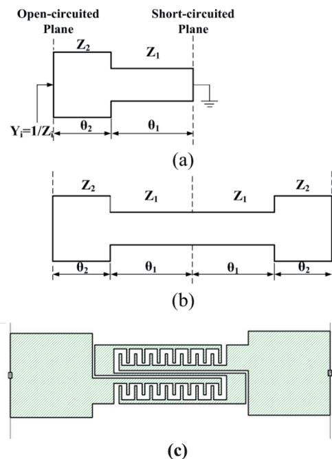
Fig. 1. The basic structures of SIR resonators: (a) Quarter-wavelength type. (b) Half-wavelength type. (c) Proposed  $\lambda/2$  structure of CISIR.
