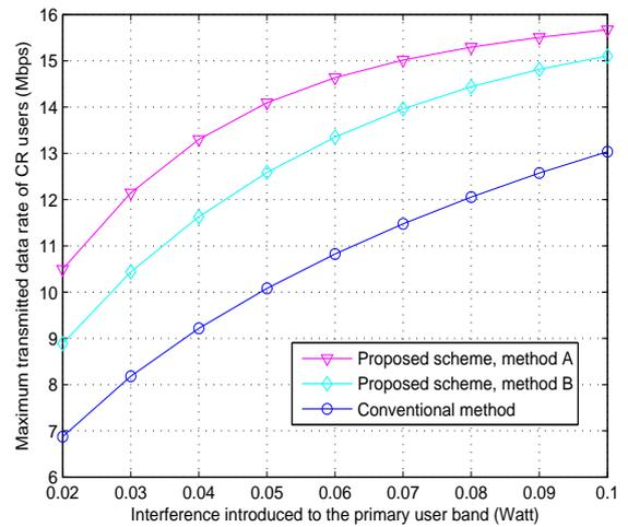
Fig. 3. Maximum CR achieved data rate versus the average interference introduced to the PU.
