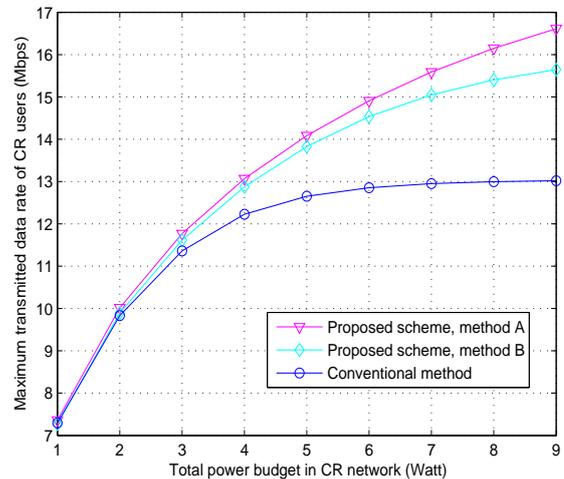
Fig. 4. Maximum CR achieved data rate versus total power budget in CR network.
