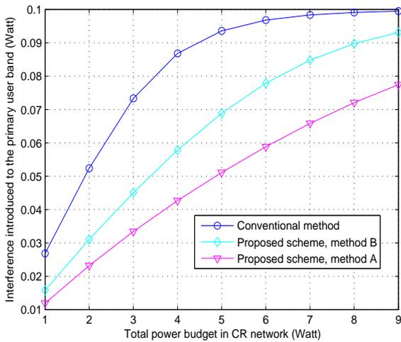
**Fig. 5.** The average interference introduced to the PU versus total power budget in CR network.
