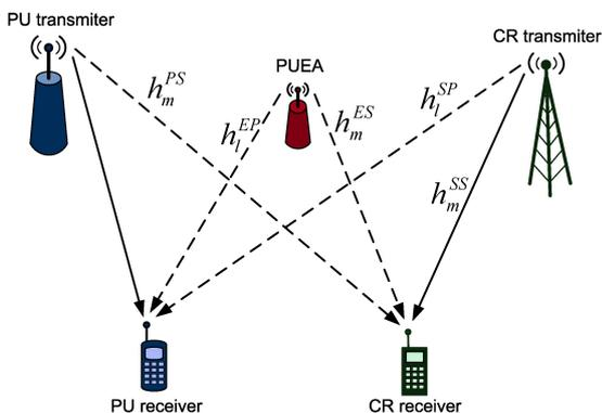
Fig. 1. System model of the considered network.
