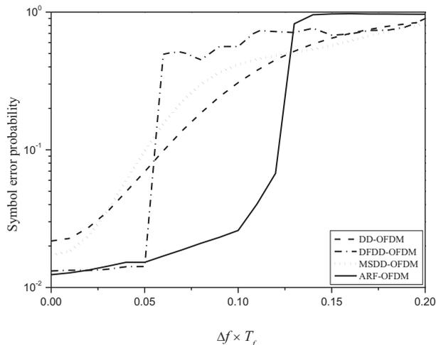
Fig. 4. Symbol error probability versus normalized frequency offset for  $N = 16$ ,  $N_{VC} = 2$  and  $T_{GI} = T_{CP} = 2T_C$ .
