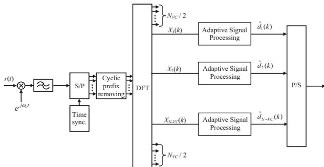
Fig. 1. ARF-OFDM receiver.
