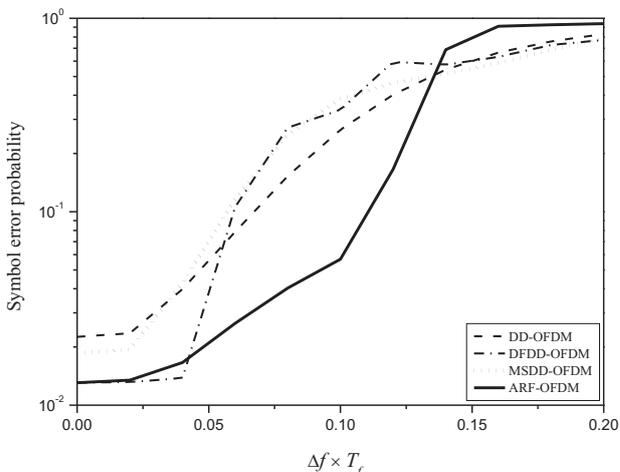
Fig. 6. Symbol error probability versus normalized frequency offset for  $N = 64$ ,  $N_{VC} = 8$  and  $T_{GI} = T_{CP} = 8T_C$ .
