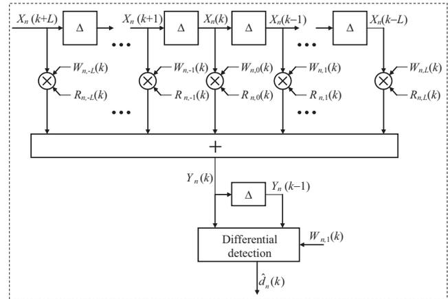
Fig. 2. Adaptive signal processing structure in  $n$ -th ARF-OFDM channel.
