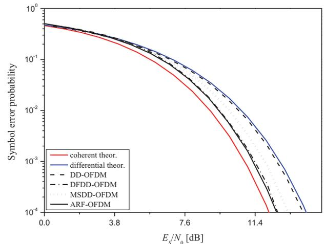
Fig. 3. Symbol error probability as function of signal to noise ratio for  $\Delta f = 0$  in AWGN channel.
