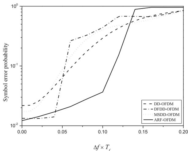
Fig. 5. Symbol error probability versus normalized frequency offset for  $N = 32$ ,  $N_{VC} = 4$  and  $T_{GI} = T_{CP} = 4T_C$ .
