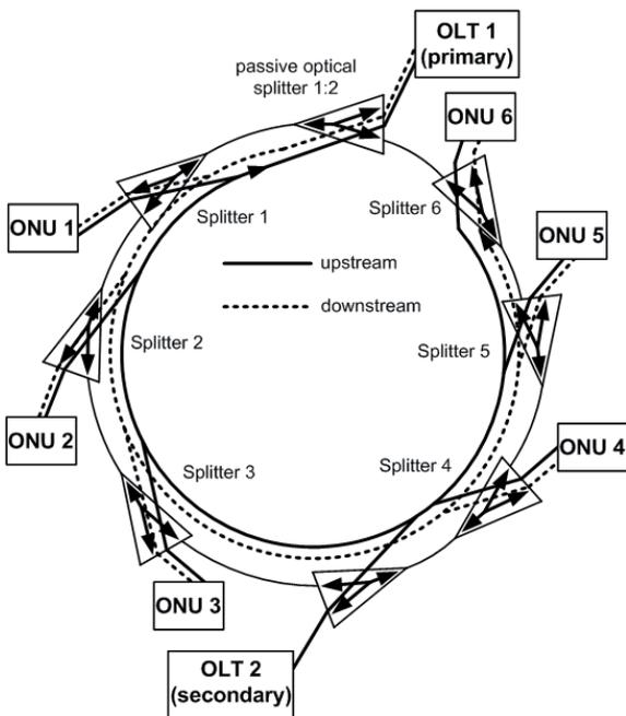
Fig. 1. The initial state of proposed ring-type PON.
