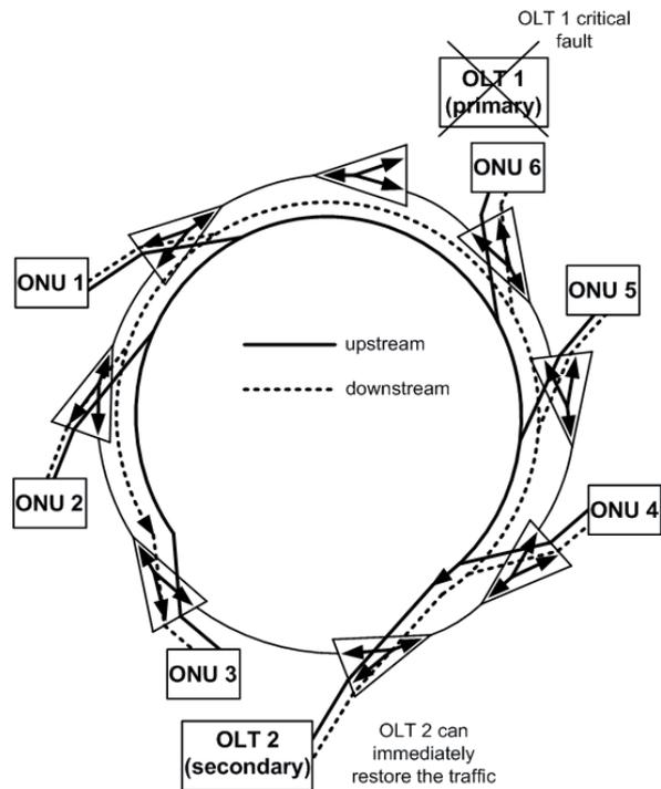
Fig. 2. Critical failure of the primary OLT unit.
