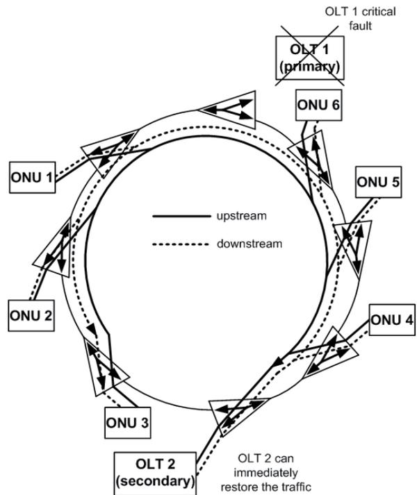
Fig. 2. Critical failure of the primary OLT unit.
