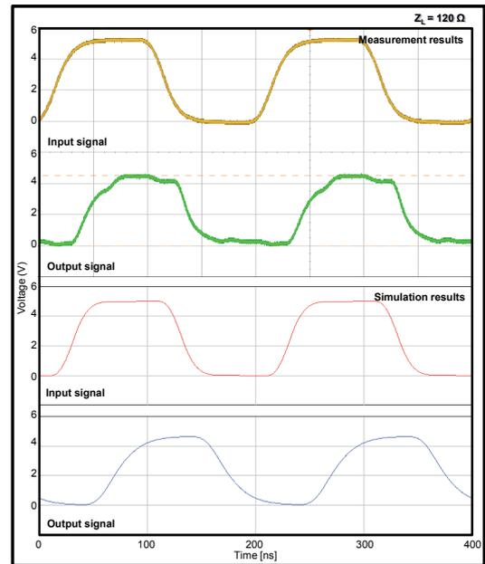
Fig. 3. Measurement vs. simulation results ( $Z_L = 120 \Omega$ ).
