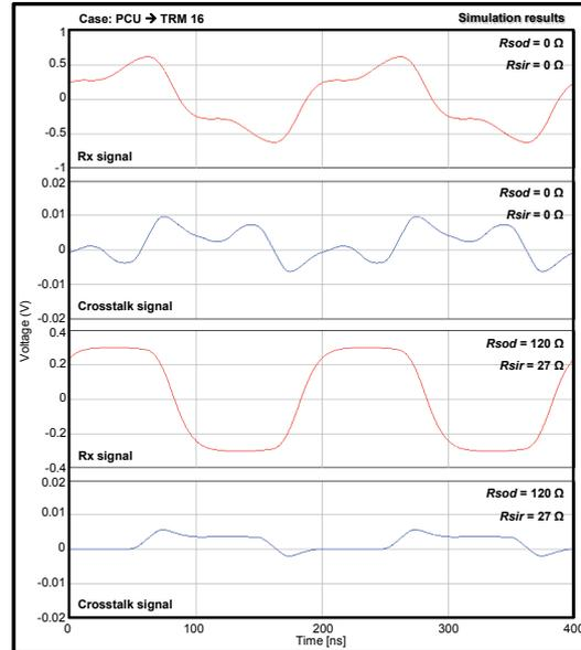
Fig. 5. Effect of serial resistors,  $R_{sod}$  and  $R_{sir}$ , on received and crosstalk voltage level (PCU → TRM 16).
