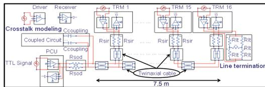
Fig. 4. Simplified electrical model which includes termination loads and serial resistors.
