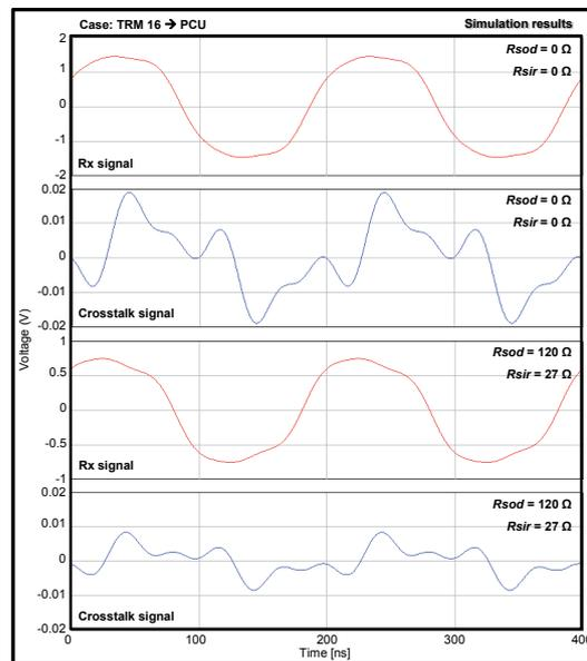
Fig. 6. Effect of serial resistors,  $R_{sod}$  and  $R_{sir}$ , on received and crosstalk voltage level (TRM 16 → PCU).
