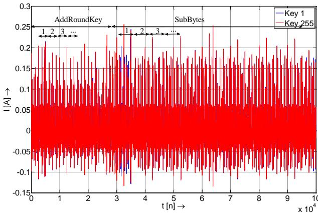
**Fig. 1.** Measured power traces for two key values.
