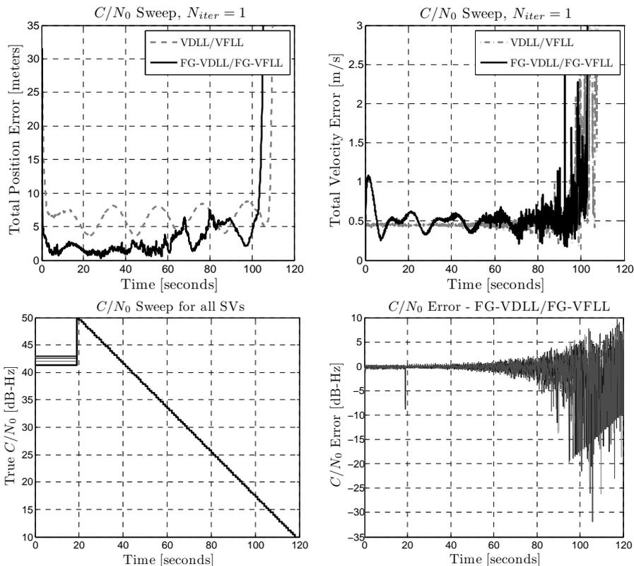
Fig. 11. Vector tracking - simulation results -  $C/N_0$  sweep. (a - upper left) TPE at  $C/N_0$  sweep, (b - upper right) TVE at  $C/N_0$  sweep, (c - lower left) swept  $C/N_0$  of all visible SVs, (d - lower right)  $C/N_0$  estimate error for all visible SVs. Figures (a-d) refer to MD,  $N_{iter} = 1$ .
