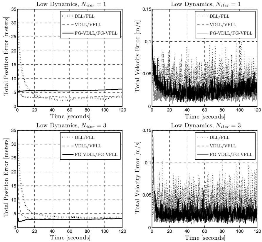
Fig. 9. Vector tracking - simulation results - LD. (a - upper left) TPE,  $N_{iter} = 1$ , (b - upper right) TVE,  $N_{iter} = 1$ , (c - lower left) TPE,  $N_{iter} = 3$ , (d - lower right) TVE,  $N_{iter} = 3$ .
