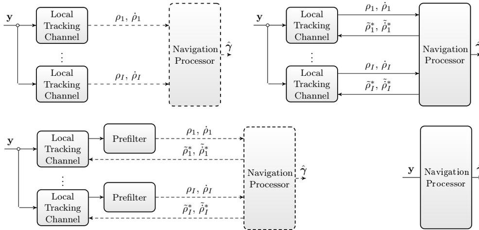
**Fig. 1.** Receiver architectures: (upper left) conventional architecture, (upper right) vector tracking architecture, (lower left) vector tracking architecture with prefilters, (lower right) direct positioning architecture. Lines denoted as dash operate at low rate (navigation update rate - typically 0.1 s or 1 s), whereas solid lines operate at much higher rate.
