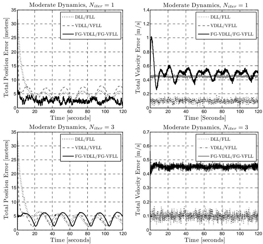
Fig. 10. Vector tracking - simulation results - MD. (a - upper left) TPE,  $N_{iter} = 1$ , (b - upper right) TVE,  $N_{iter} = 1$ , (c - lower left) TPE,  $N_{iter} = 3$ , (d - lower right) TVE,  $N_{iter} = 3$ .
