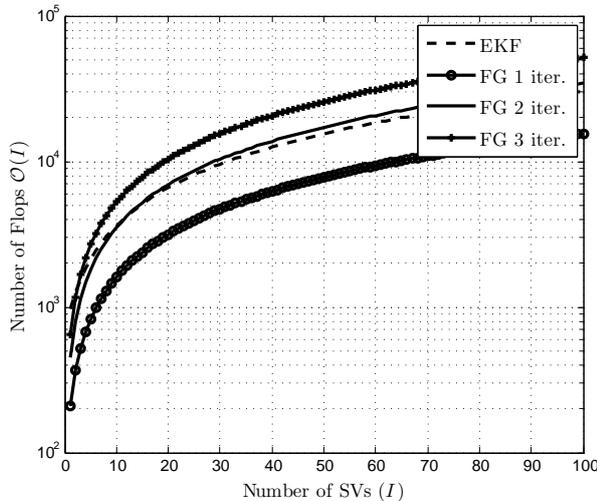
Fig. 6. Complexity comparison of the PVT filtering algorithms. Symbol  $O(I)$  denotes the number of floating point operations (flops) depending on the number of SVs denoted as  $I$ .
