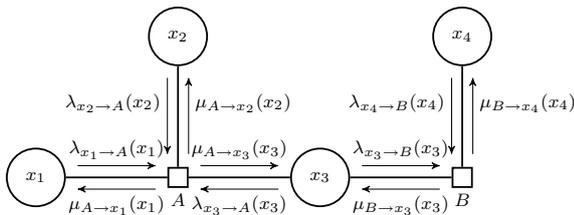
**Fig. 2.** Example FG with MP for global function  $p(x_1, x_2, x_3, x_4)$  that factors into local functions  $p_A(x_1, x_2, x_3), p_B(x_3, x_4)$  in the following manner  $p(x_1, x_2, x_3, x_4) = p_A(x_1, x_2, x_3) \cdot p_B(x_3, x_4)$ . The direction of the messages is denoted with arrow.
