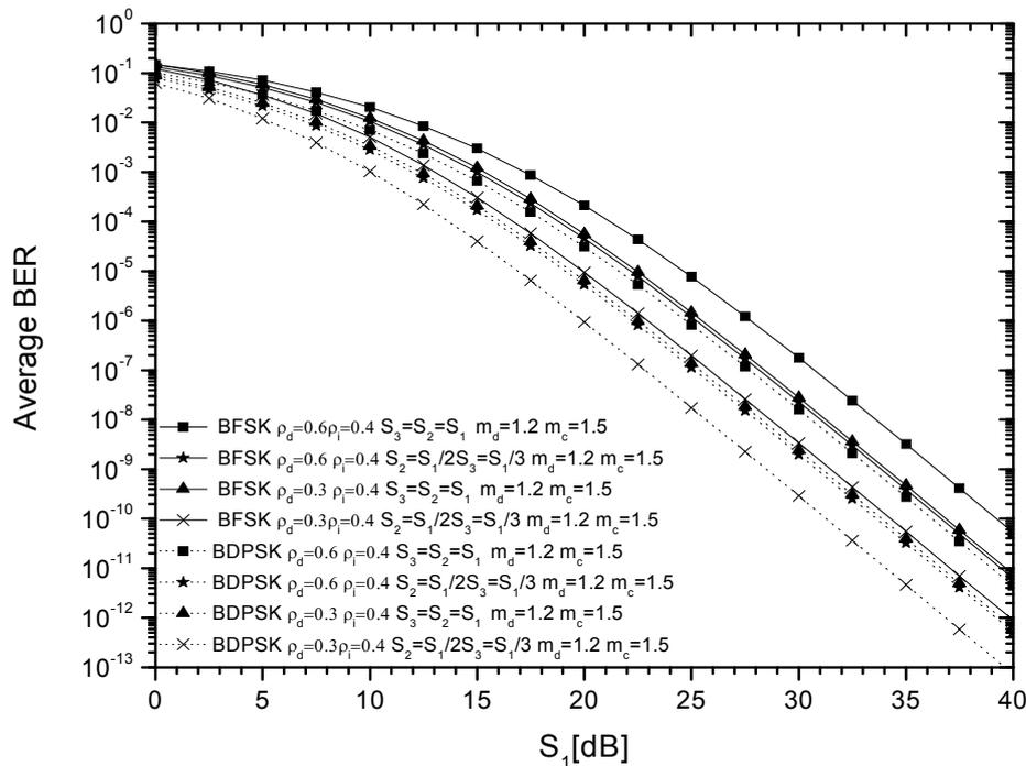
Fig. 2. Average BER versus  $S_1$  in noncoherent BDPSK and BFSK.
