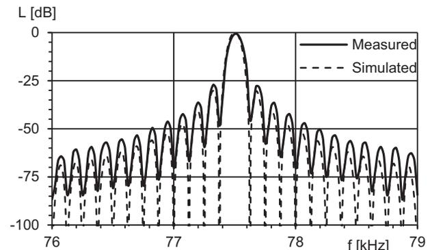
Fig. 11. Measured characteristic of implemented filter.
