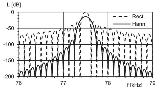
Fig. 9. Windowing influence on the frequency characteristic.
