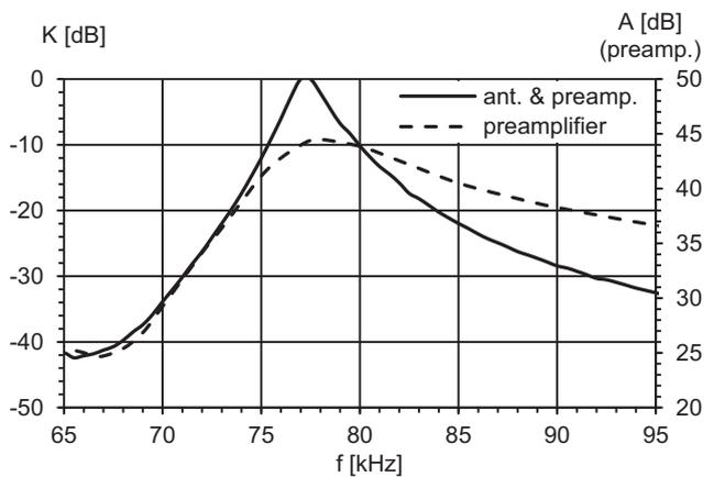
Fig. 5. Measured frequency response of the prototype.
