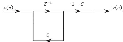
Fig. 15. Signal diagram of averager.
