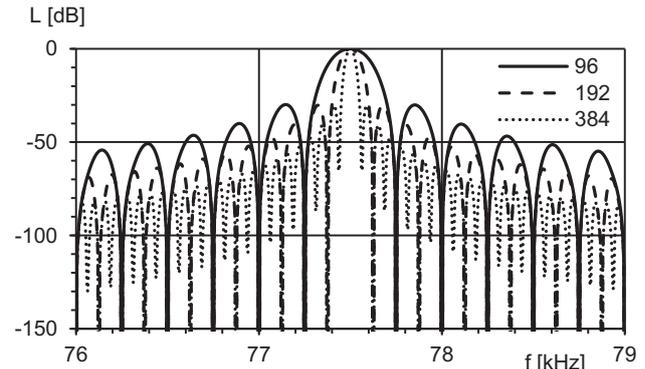
Fig. 10. Frequency responses of filters of different lengths.
