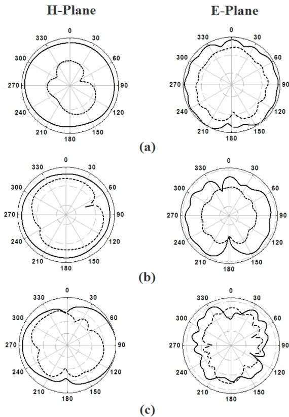
Fig. 13. Measured co-polarized (solid line) and cross-polarized (dashed line) patterns of the antenna: (a) 3.1 GHz, (b) 6.8 GHz, (c) 9 GHz.
