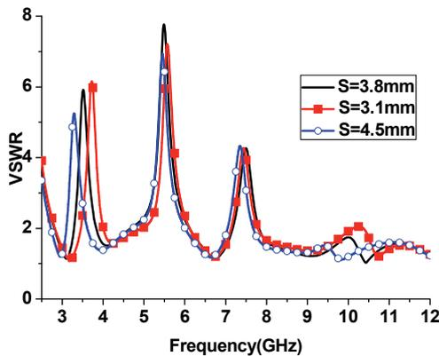
Fig. 5. Simulated band-notched characteristics of the proposed antenna for various  $S$ .
