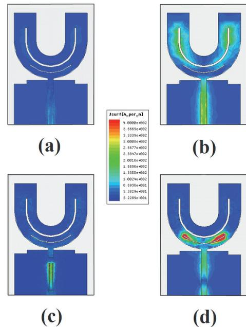
Fig. 8. Surface current distributions of the antenna. (a) A pass-band at 6.8 GHz. (b) The first notched band at 3.5 GHz. (c) The second notched band at 5.5 GHz. (d) The third notched band at 7.5 GHz.
