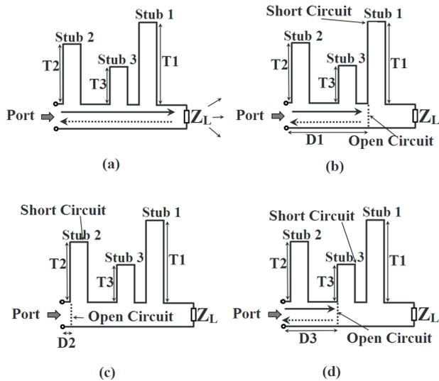
Fig. 9. The distributed element equivalent circuit. (a) At the pass-band. (b) The first notched band at 3.5 GHz. (c) The second notched band at 5.5 GHz. (d) The third notched band at 7.5 GHz.
