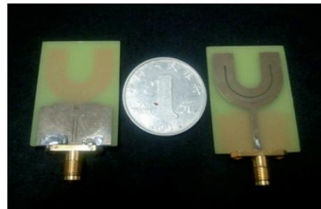
Fig. 3. Photograph of the fabricated antenna.
