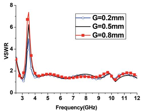
Fig. 2. Effects of  $G$  (the width of slot S1).
