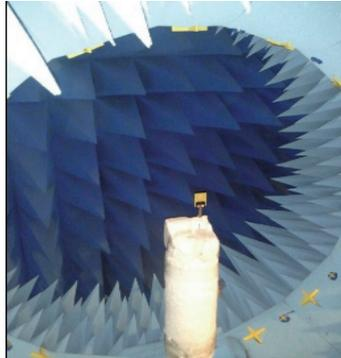
Fig. 12. Photograph of the proposed antenna in an anechoic chamber.
