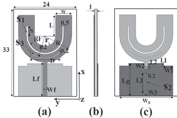
Fig. 1. Geometry of the antenna (units in millimeters). (a) Top view. (b) Side view. (c) Bottom view.
