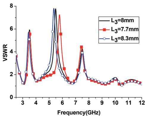
Fig. 6. Simulated band-notched characteristics of the proposed antenna for various  $L_3$ .
