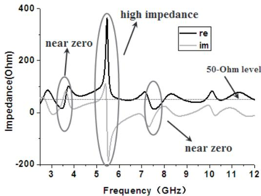
Fig. 10. Input impedance of proposed antenna.
