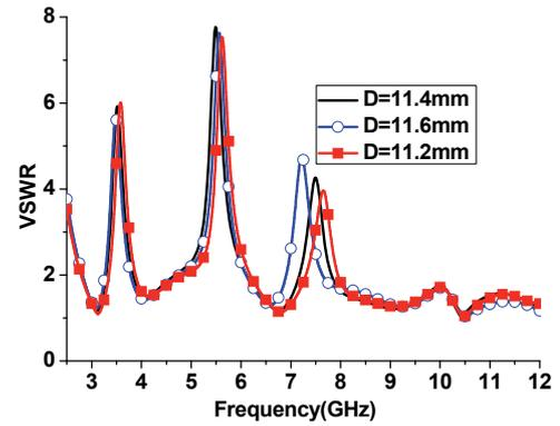
Fig. 7. Simulated band-notched characteristics of the proposed antenna for various  $D$ .
