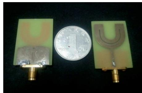
Fig. 3. Photograph of the fabricated antenna.
