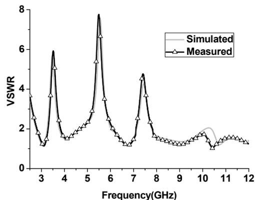
Fig. 11. Measured and simulated VSWR for antenna.
