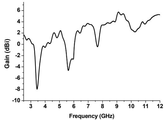
Fig. 14. Measured gain of the proposed antenna with triple band-notched characteristics.
