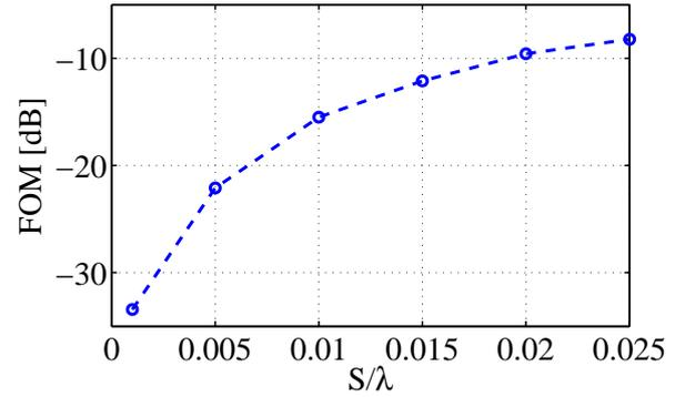
**Fig. 4.** Figure of merit to calculate the deviations between the presented equations and the FIT for different feeding width.  $L = 225$  mm,  $W = 20$  mm, operating frequency = 300 MHz.
