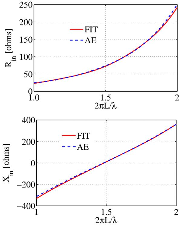
**Fig. 2.** Real (top) and imaginary (bottom) parts of the input impedance of a strip dipole antenna as a function of frequency calculated by the Finite Integration Technique (FIT) and by the novel Analytical equations (AE).  $\frac{2\pi L}{\lambda} = 1.5$ ,  $\frac{W}{\lambda} = 0.003$ ,  $\frac{S}{\lambda} = 0.002$ , central frequency = 600 MHz.
