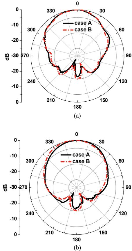
Fig. 7. Measured radiation patterns: (a) E-plane, (b) H-plane.
