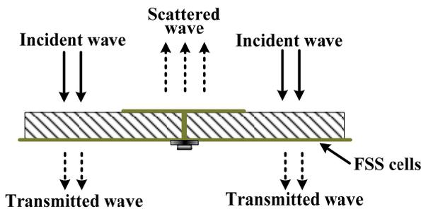
Fig. 1. RCS reduction schematic.
