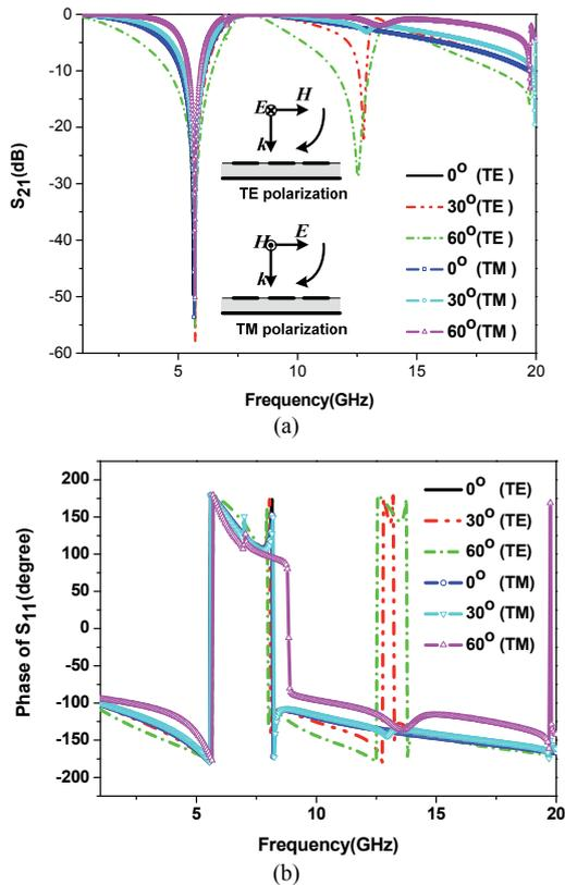
Fig. 3. Numerical results under different incidence angles: (a) transmission coefficients, (b) reflection phases.
