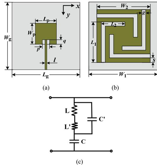
Fig. 2. (a) Geometry of microstrip patch antenna. (b) Geometry of designed FSS unit cell. (c) Equivalent circuit model of designed FSS.
