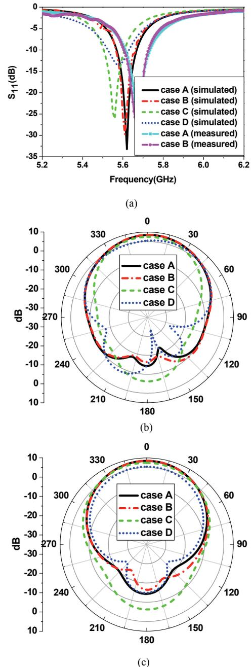
Fig. 5. Comparison among radiation performance with different cases: (a) reflection coefficients, (b) simulated radiation patterns in E-plane, (c) simulated radiation patterns in H-plane.
