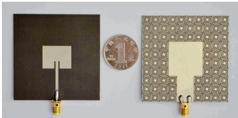
Fig. 6. Top and bottom views of the fabricated patch antenna.
