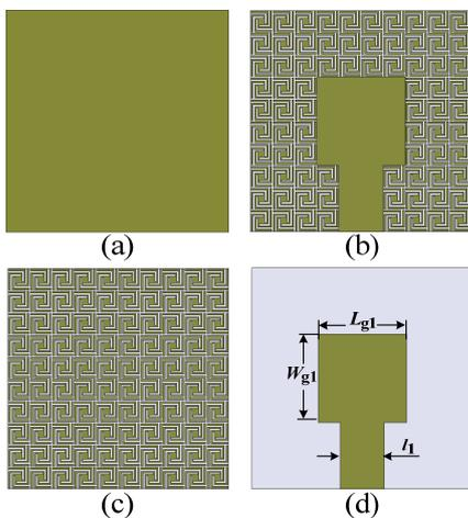
Fig. 4. Different patterns of antenna ground: (a) case A, (b) case B, (c) case C, (d) case D.
