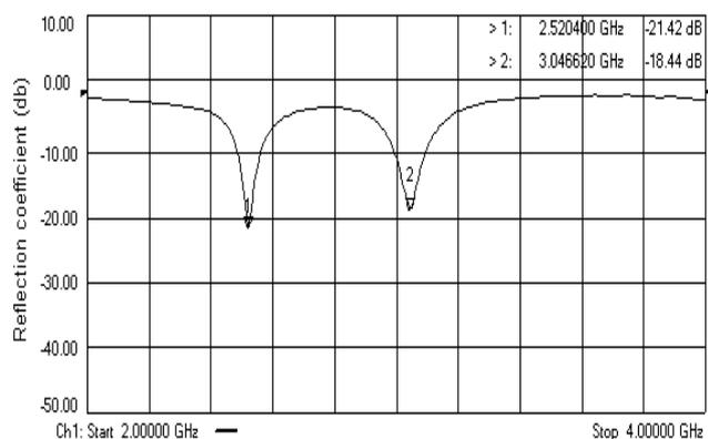
Fig. 2. Measured variation of reflection coefficient with frequency for the single layer modified rectangular patch antenna.
