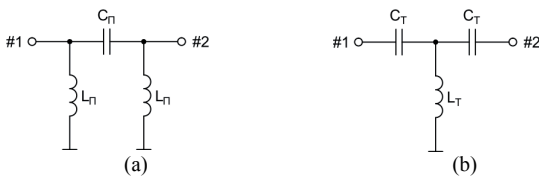
Fig. 10. Two investigated structures of the high-pass LC networks as artificial left-handed transmission lines: Pi-shaped (a) and T-shaped (b).
