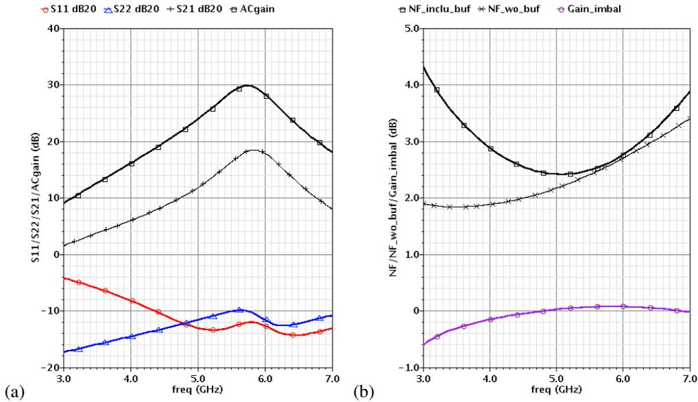
Fig. 8. Simulated s-parameters  $S_{21}$ ,  $S_{11}$ ,  $S_{22}$  (a), noise figure NF and gain imbalance (b) for highest gain and band settings. The measurement buffer loss is de-embedded for  $S_{21}$  and NF.
