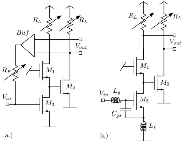
**Fig. 1.** Balun LNA topologies based on buffered resistive feedback (a) and inductive source degeneration input (b).
