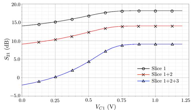
**Fig. 7.** Simulated small-signal gain ( $S_{21}$ ) in dependence on the gain control voltage  $V_{C1}$  for the 3 slices.
