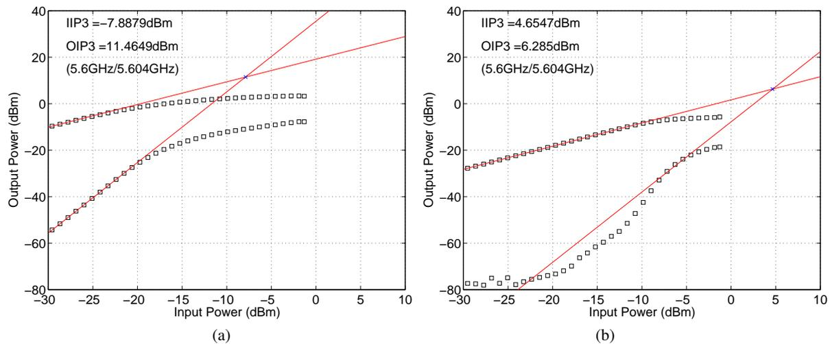
**Fig. 13.** Measured LNA IIP3 for the highest gain and highest band setting (a) and for the lowest gain and highest band setting (b). The measurement buffer loss is de-embedded.
