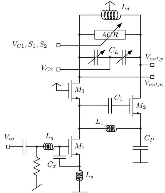
**Fig. 6.** LNA with tunable gain, where  $V_{C1}$  is the gain tuning control voltage for the active resistor (ACR),  $S_1, S_2$  are digital gain control signals and  $V_{C2}$  is the control voltage for band setting
