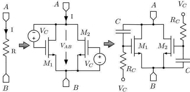
**Fig. 2.** Tunable active resistor (ACR) concept for  $R_L$  with linearity optimized MOS resistors and quasi floating gate implementation.
