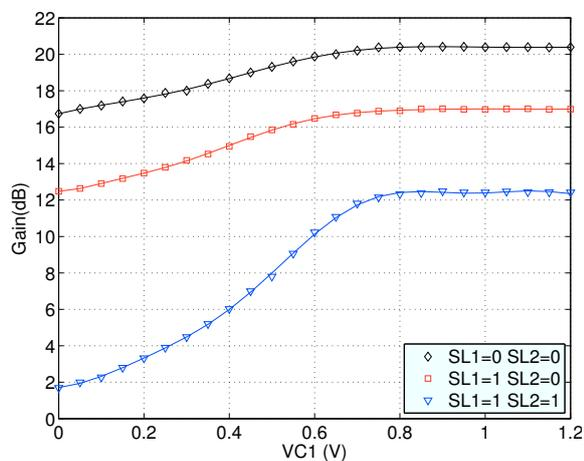
Fig. 11. Measured LNA gain tuning characteristics in dependence on control voltage  $V_{C1}$  and ACR slice enable settings.
