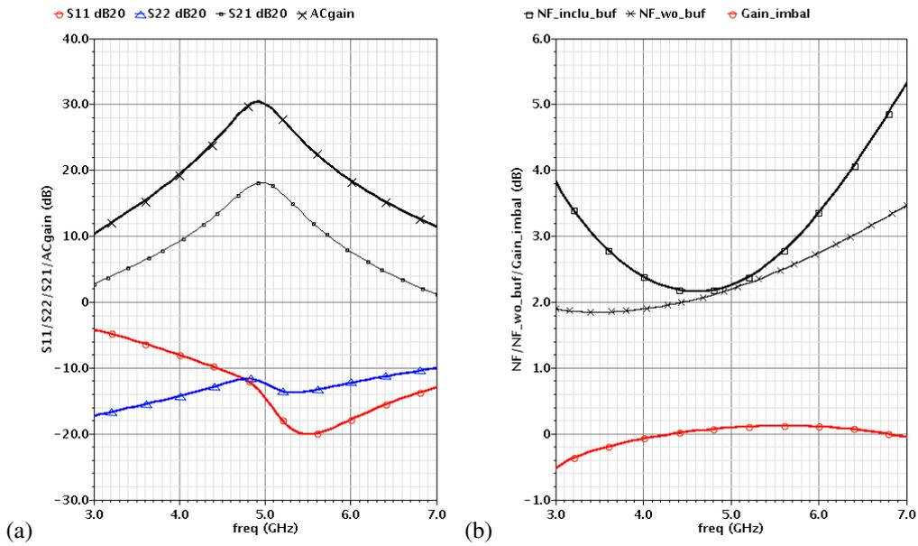
Fig. 9. Simulated s-parameters  $S_{21}$ ,  $S_{11}$ ,  $S_{22}$  (a), noise figure NF and gain imbalance (b) for highest gain and lowest band settings. The measurement buffer loss is de-embedded for  $S_{21}$  and NF.
