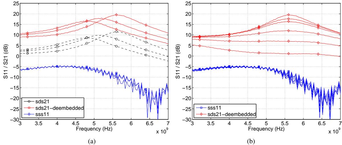
**Fig. 12.** Measured s-parameters  $S_{21}$  and  $S_{11}$  for different band-settings at the highest gain (a) and for different gain-settings at the highest frequency band (b). The measurement buffer loss is de-embedded.
