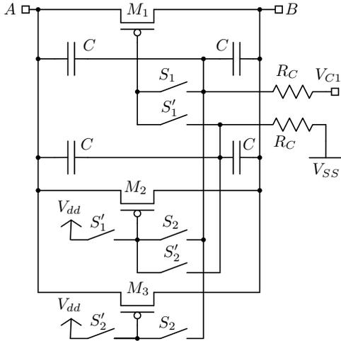
**Fig. 3.** Active resistor implementation with 3 parallel slices to increase tuning range. The slices are enabled via switches  $S_1, S_2$  and the resistance is controlled by an analog control voltage  $V_{C1}$ , tunable between 0 V and  $V_{dd}$ .
