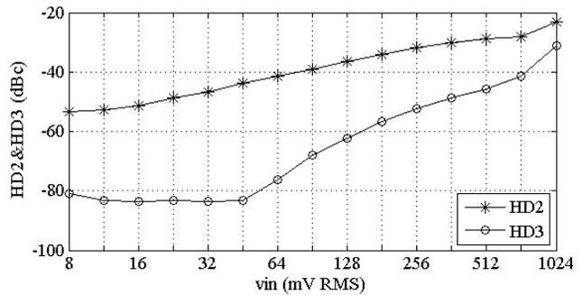
**Fig. 5.** Measurement results of 2<sup>nd</sup> order (HD2) and 3<sup>rd</sup> order (HD3) harmonic distortion for active resistor (ACR) in dependence on the signal level.
