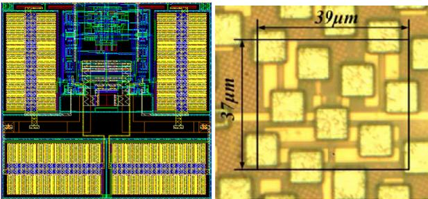
**Fig. 4.** Active resistor layout (left) and photograph (right).
