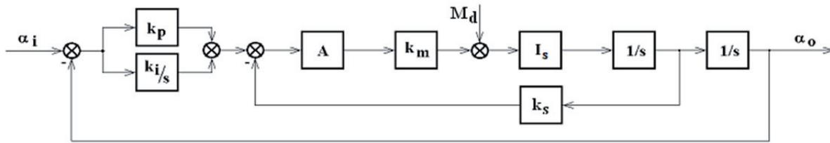
Fig. 3. Block diagram of the MFSO station servomechanisms.
