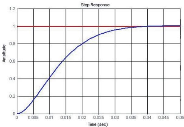
Fig. 4. Servo's response to the unit step input.
