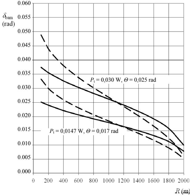
**Fig. 2.** Angular deviation limits of the Gaussian (---) and the Top Hat beam (-) - considering atmospheric interference.
