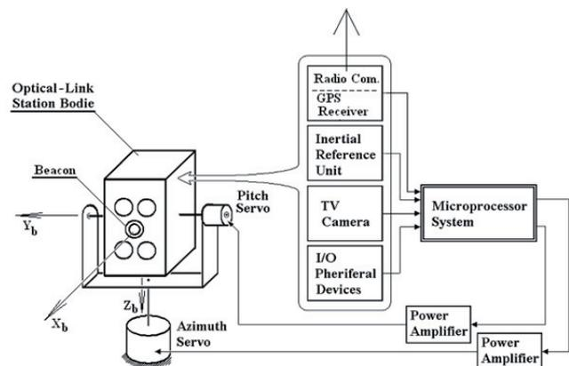
Fig. 1. Structure of a moving FSO station.
