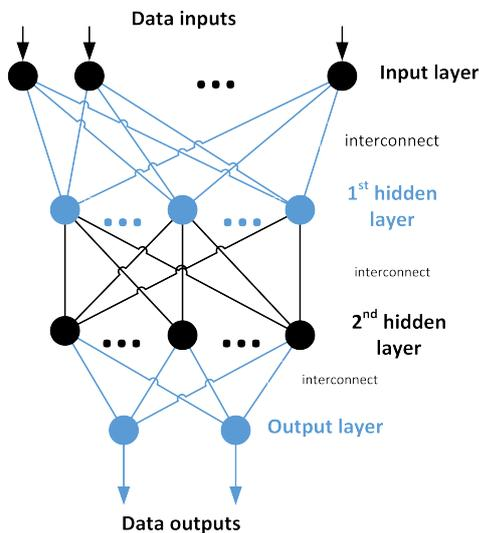
Fig. 1. Typical architecture of a fully connected feed-forward ANN used for data processing in this article.
