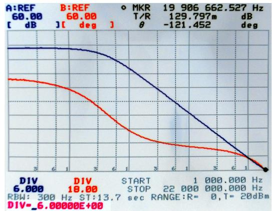
Fig. 10. Measured magnitude and phase responses in closed-loop configuration.
