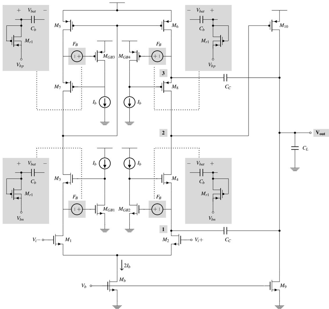
Fig. 2. Floating Battery Gain-Boosted Telescopic Amplifier (FBGBTA).
