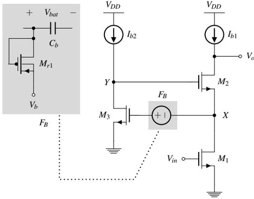
Fig. 1. Floating battery gain-boosted telescopic amplifier (FBGBTA).
