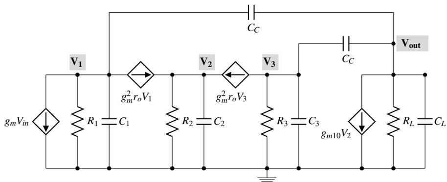
Fig. 3. Small signal model of the Two-Stage Amplifier.
