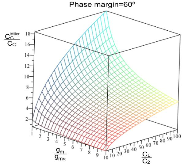
Fig. 4. Reduction of  $C_C$  respect Miller compensation.
