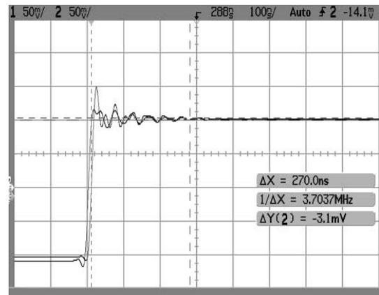
Fig. 11. Experimental step response for a non-inverting unity-gain configuration.
