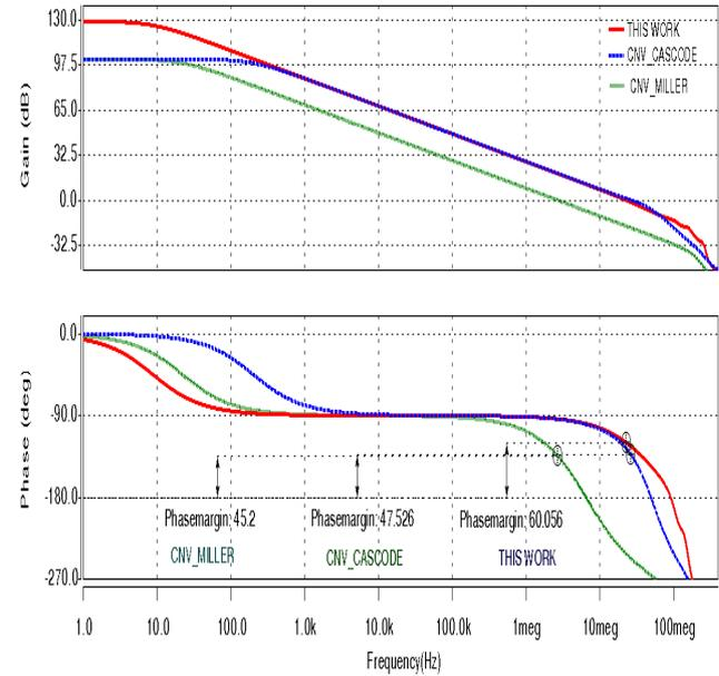
Fig. 6. Frequency response of Proposed, Conventional Cascode and conventional Miller two stage amplifiers with  $C_L = 45 \text{ pF}$ .
