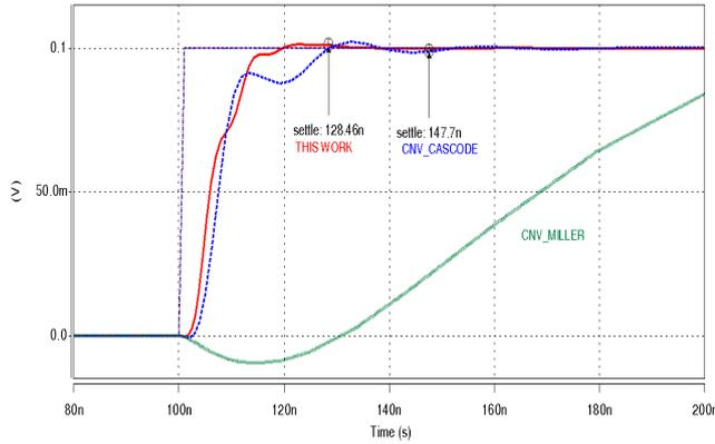
Fig. 7. Settling time simulation results.
