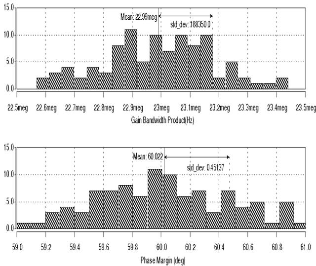
Fig. 8. Phase Margin Monte Carlo simulation
