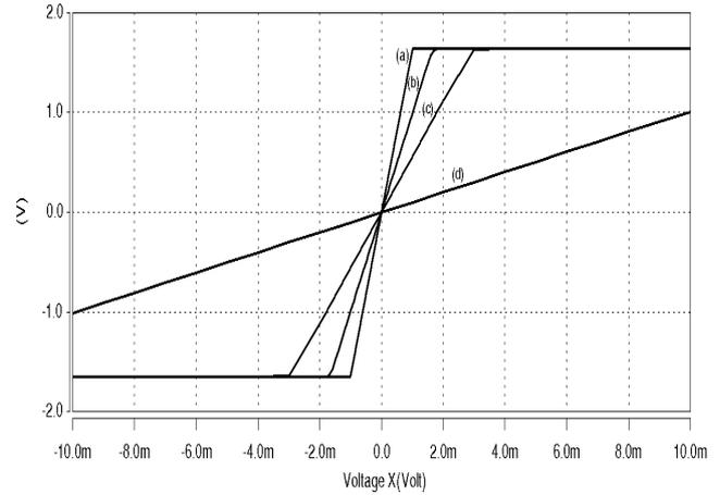
Fig. 5. Input Output DC transfer characteristic for a) 74 dB Gain, b) 60 dB Gain, c) 54.9 dB and d) 40 dB
