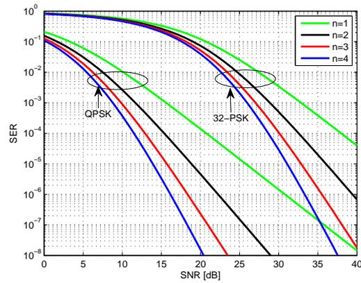
Fig. 7. SER versus SNR with (1, 2, 3 and 4) relays using QPSK and 32PSK modulation signals.
