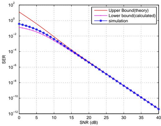
Fig. 4. Comparison of an upper bound and lower bound with simulation using QPSK signal for a one-relay system.
