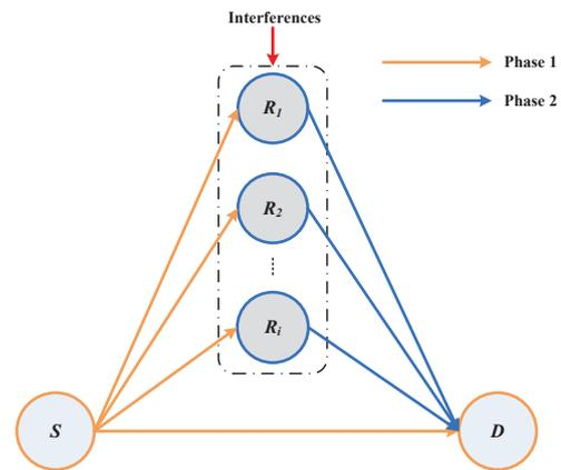
Fig. 2. Cooperation model with interferences at relay nodes.
