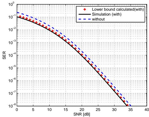
Fig. 5. Representation of SER using QPSK modulation for lower bound (calculated) and simulation curves compared with best AF-DF protocol with no interference.
