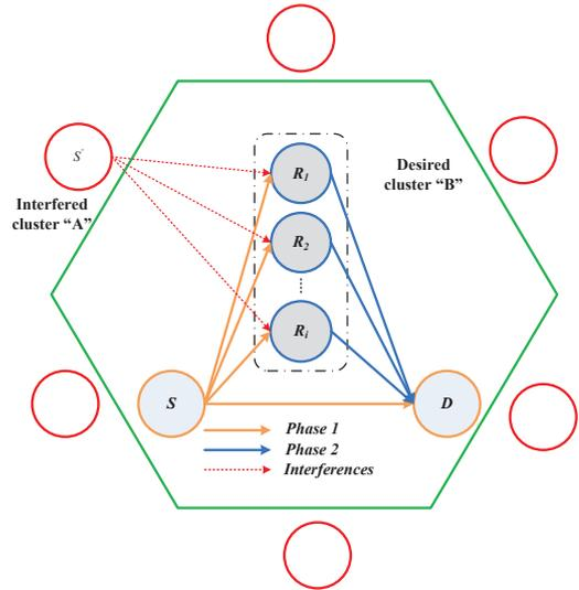
Fig. 1. Cooperative relaying protocol selection between AF and DF, where the continuous lines refer to the required channels and the dashed lines represent the interference channels.
