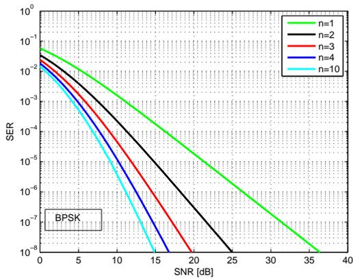
Fig. 6. Symbol error rate for BPSK signals.
