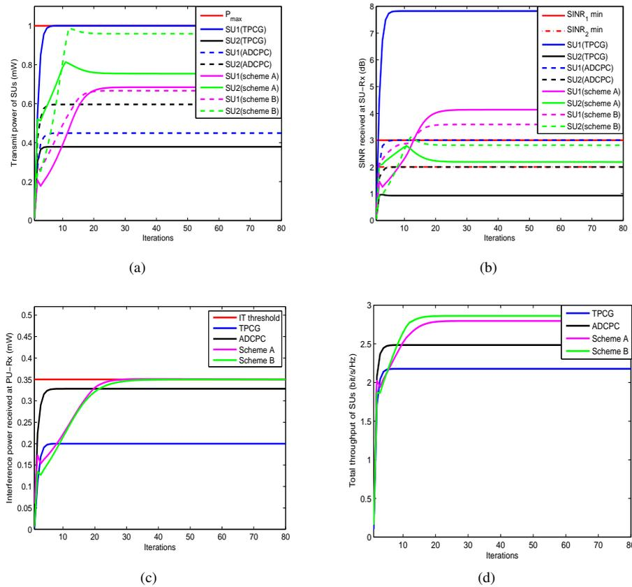
**Fig. 3.** Performance comparisons between the proposed algorithms and the existing algorithms; (a) Transmit power of SUs. (b) Received SINRs of SUs. (c) Aggregated interference power at PU-Rx. (d) Total throughput of system.
