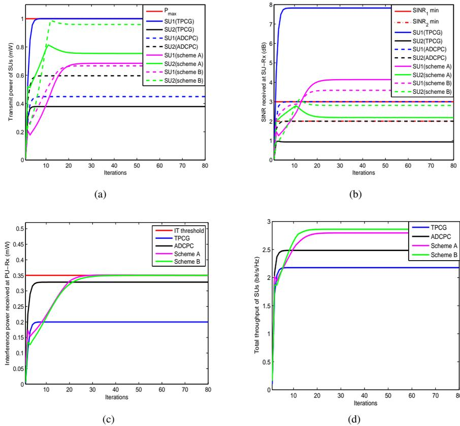
**Fig. 3.** Performance comparisons between the proposed algorithms and the existing algorithms; (a) Transmit power of SUs. (b) Received SINRs of SUs. (c) Aggregated interference power at PU-Rx. (d) Total throughput of system.
