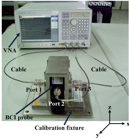
Fig. 1. Experimental setup for calibrating the transfer impedance of BCI probe using the calibration fixture.
