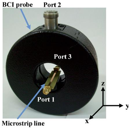
Fig. 6. Experimental setup for measuring the common-mode conversion coefficient of the microstrip lines with different ground planes.
