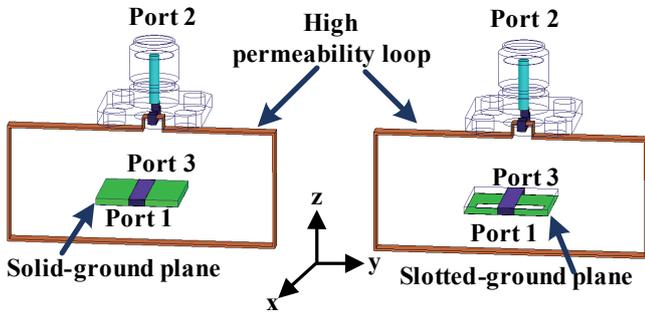
Fig. 7. EM simulation configuration for obtaining the common-mode conversion coefficient of the microstrip lines with different ground planes. (a) Solid ground plane. (b) Slotted ground plane.
