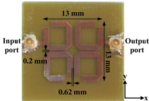
Fig. 10. Top view dimensions of four-order microstrip quasi-elliptic bandpass filter implemented on the FR4 substrate.
