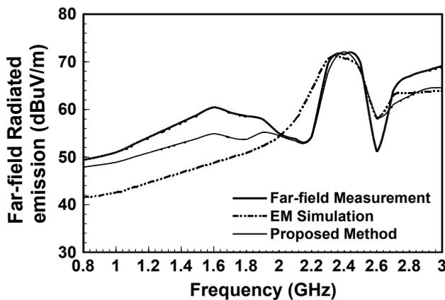
Fig. 16. Comparison of radiated emissions from the microstrip bandpass filter obtained in a fully-anechoic chamber with predictions by the proposed method and EM simulation.
