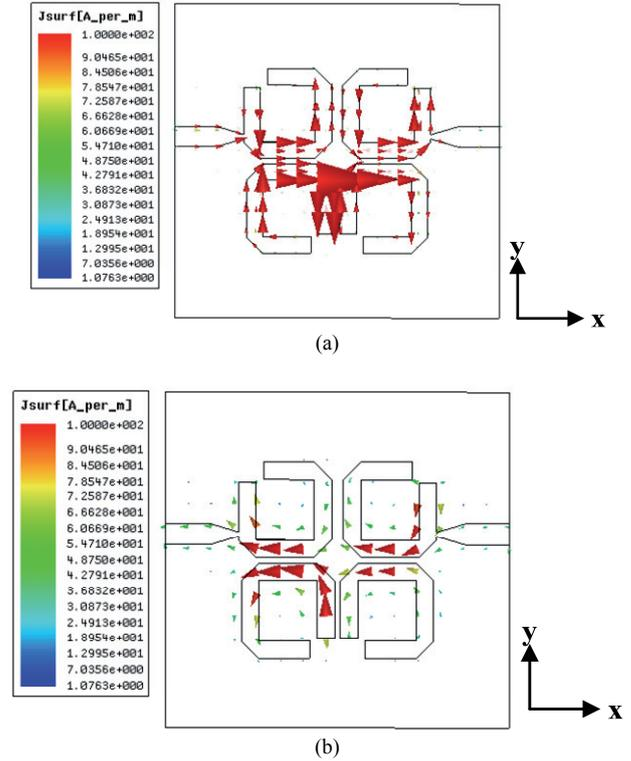
Fig. 12. Simulated surface current density distribution of microstrip bandpass filter at the frequency of 2.4 GHz. (a) Signal trace. (b) Ground plane.
