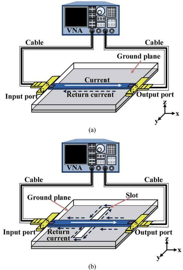
Fig. 5. Radiated emissions caused by a microstrip line with different ground planes. (a) Solid ground plane. (b) Slotted ground plane.
