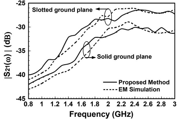
Fig. 8. Comparison of common-mode conversion coefficient magnitudes of the microstrip line with different ground planes between the proposed method and EM simulation.
