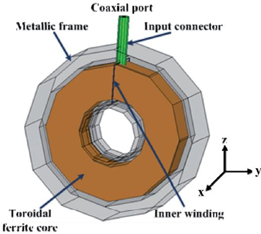
Fig. 2. Geometrical configuration of the BCI probe.
