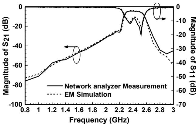
Fig. 11. Comparison of return loss and insertion loss of the microstrip bandpass filter between network analyzer measurement and EM simulation.
