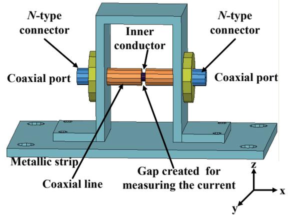
Fig. 3. Geometrical configuration of the calibration fixture.
