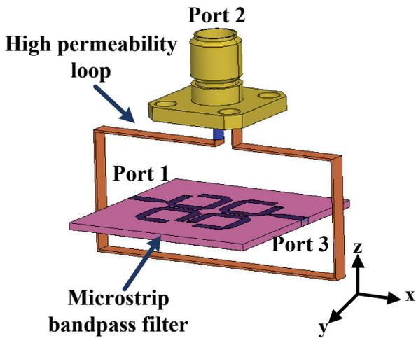
Fig. 14. EM simulation configuration for obtaining the common-mode conversion coefficient of the microstrip bandpass filter.
