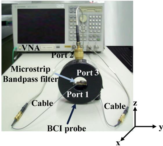
Fig. 13. Experimental setup for measuring the common-mode conversion coefficient of the microstrip bandpass filter.
