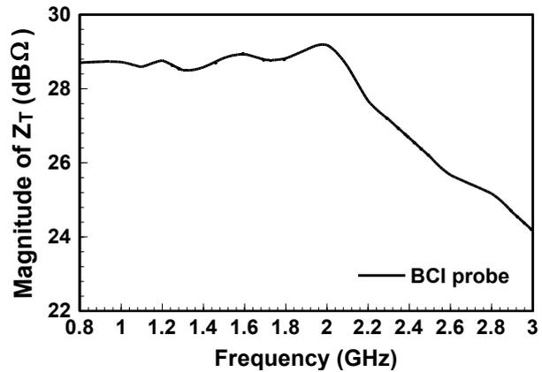
Fig. 4. Magnitude of the BCI probe transfer impedance by using the calibration setup shown in Fig. 1.
