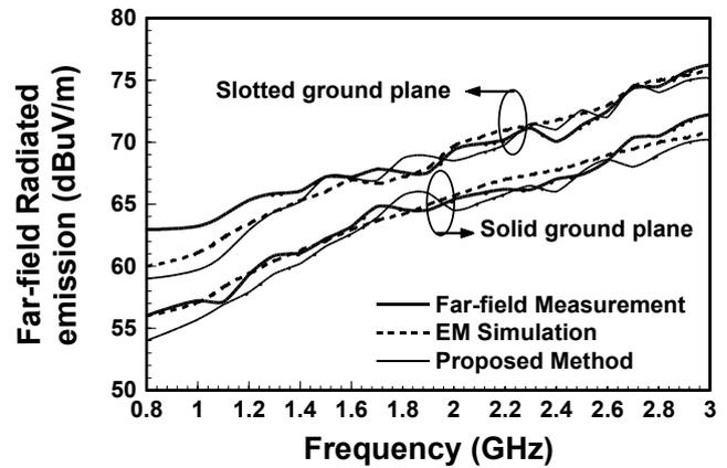
Fig. 9. Comparison of far-field radiated emissions from the microstrip line with different ground planes obtained in a fully-anechoic chamber with predictions by the proposed method and EM simulation.
