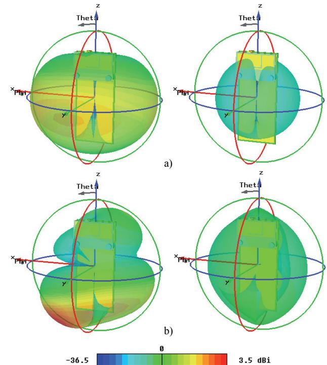
Fig. 4. Simulated radiation patterns at a) 925 MHz and b) 1795 MHz of the PIFA. Left pictures represent vertically polarized waves, the right pictures are computed for horizontally polarized waves.
