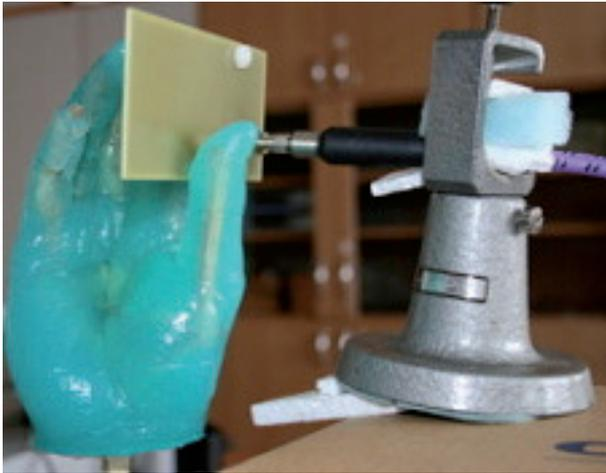
Fig. 7. Photo of the phantom prototype during antenna impedance match measurement.
