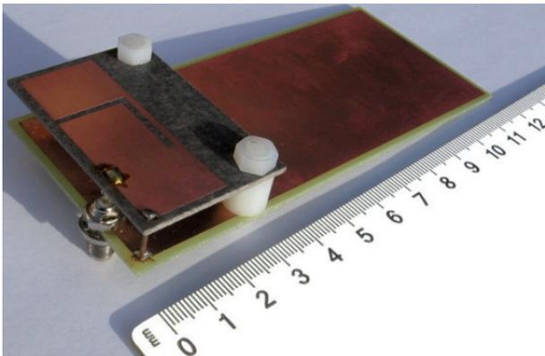
Fig. 2. Photo of the dual-band PIFA prototype.
