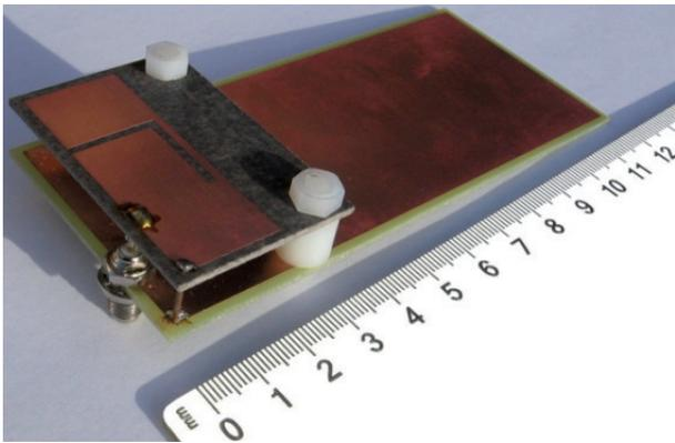
Fig. 2. Photo of the dual-band PIFA prototype.
