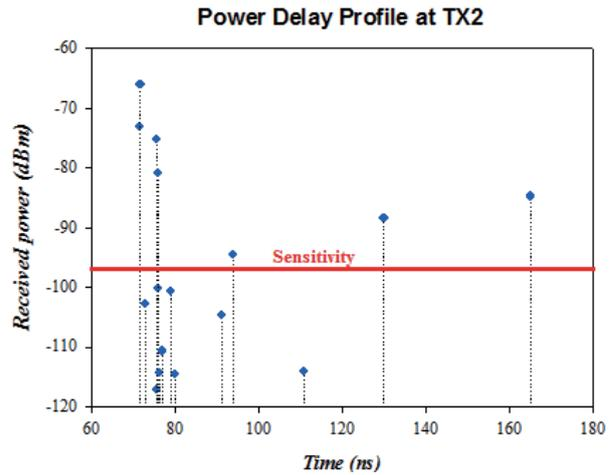
Fig. 8. Power Delay Profile at location of TX2 (the farthest node), while TX1 is transmitting.
