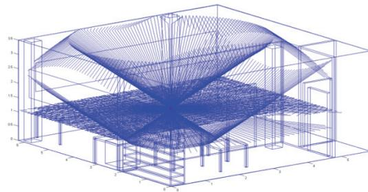
Fig. 4. Schematic of 3D ray launching within an indoor scenario.
