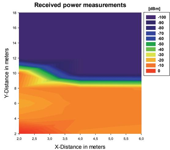
Fig. 17. Measured power levels in dBm for a pair of mote coordinator/sensor in the indoor scenario at highest transmission data rate.
