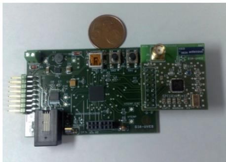
Fig. 2. Image of the main board (left) and the radio frequency module (right) of the mote device.
