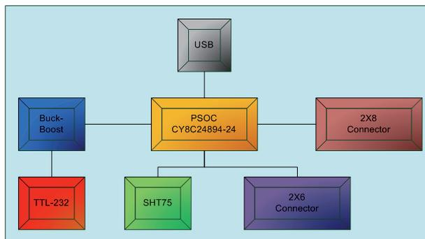
Fig. 1. Block diagram for the implemented mote device.
