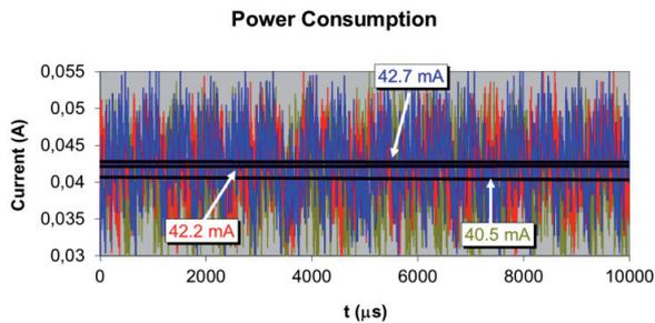
**Fig. 19.** Detail on the power consumption for the designed mote device within the indoor scenario. The mean values for different currents are proportional to the separation between motes.
