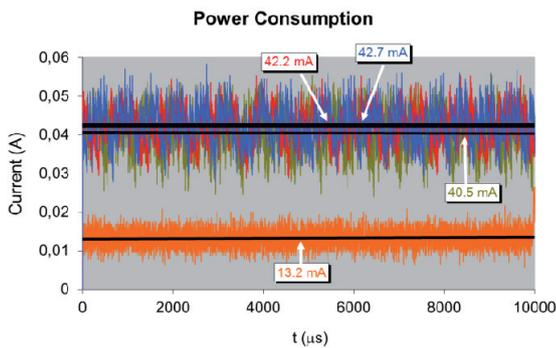
**Fig. 18.** Power consumption variation as a function of time for different positions. The bottom curve (13.2 mA) is for standby, whereas as the rest of the curves span from the closest to the farthest mote within the measurement scenario.
