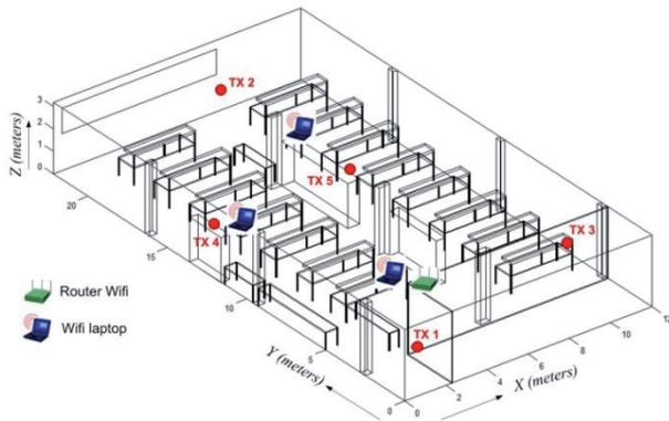
Fig. 11. Schematic representation of the scenario used to calculate the SNR planes of Fig. 12.
