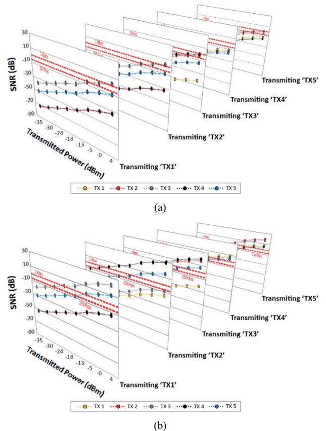
Fig. 13. SNR values at each CyFi mote position for a single transmitting mote, while WiFi-interference sources are transmitting (a) 20 dBm and (b) 0 dBm.
