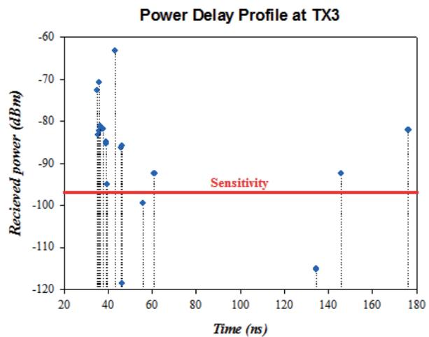
Fig. 9. Power Delay Profile at location of TX3 (the nearest node), while TX1 is transmitting.
