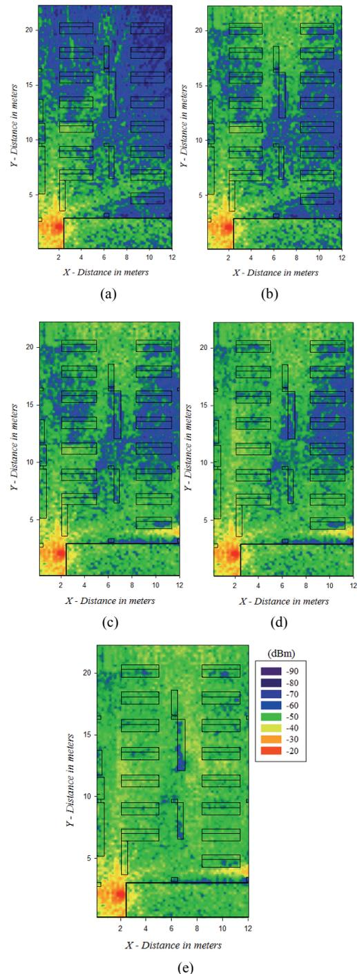
**Fig. 6.** RSSI 3D ray launching simulation results obtained at a bidimensional plane at a height of 0.81 m for different number of transmitters: (a) TX 1, (b) TX1 and TX2, (c) TX1, TX2 and TX 3, (d) TX1, TX2, TX3 and TX4, (e) TX1, TX2, TX3, TX4 and TX5.
