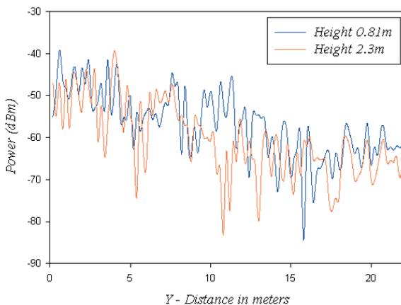
Fig. 7. Simulation results for height 0.81 m and height 2.3 m, for X = 3.5 m, along the Y-axis of the indoor scenario under analysis.
