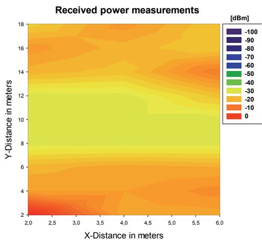
Fig. 16. Measured power levels in dBm for a pair of mote coordinator/sensor in the indoor scenario.
