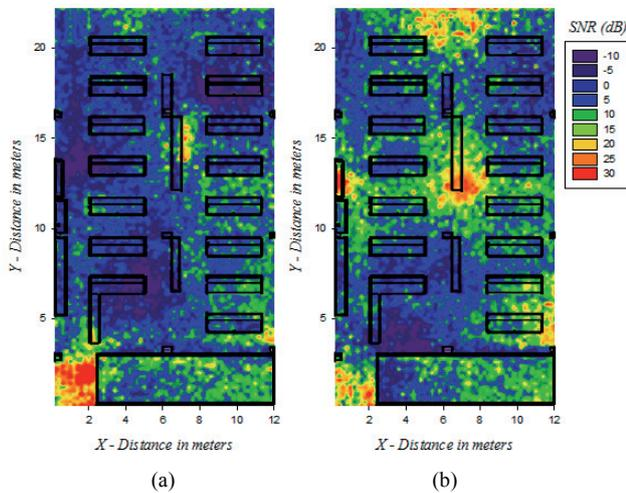
Fig. 12. Spatial distribution of signal to noise ratio in the indoor scenario of Fig. 5 for two different heights: (a) 0.81 meters, (b) 2.3 meters.
