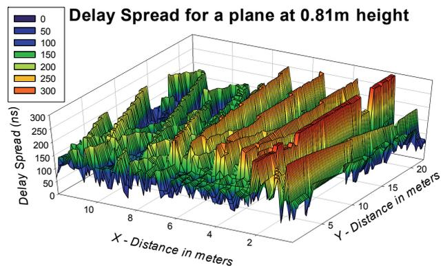
Fig. 10. Delay Spread values for a plane at 0.81 meters height (i.e. the height of TX1 within the scenario).
