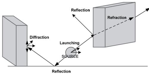
Fig. 3. Principle of Ray Launching method.
