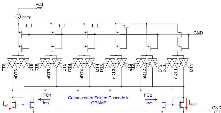
Fig. 3. M-2M converting network.
