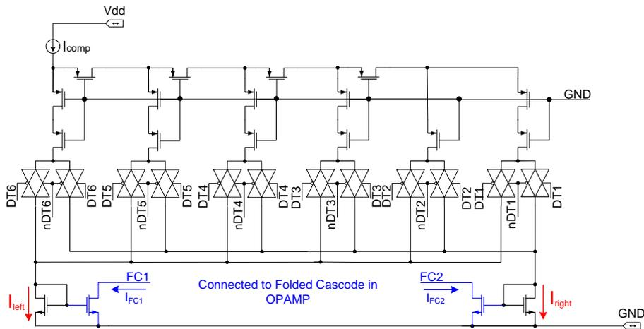
Fig. 3. M-2M converting network.
