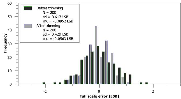
Fig. 11. Deviation of the full scale error.
