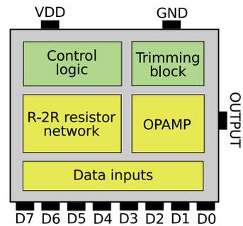
Fig. 1. Block diagram of the self-calibrated R-2R DAC.
