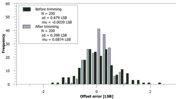
Fig. 9. Deviation of the offset error.
