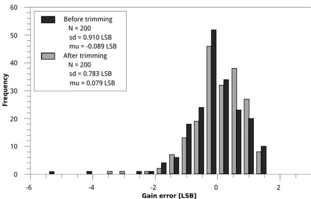
Fig. 10. Deviation of the gain error.
