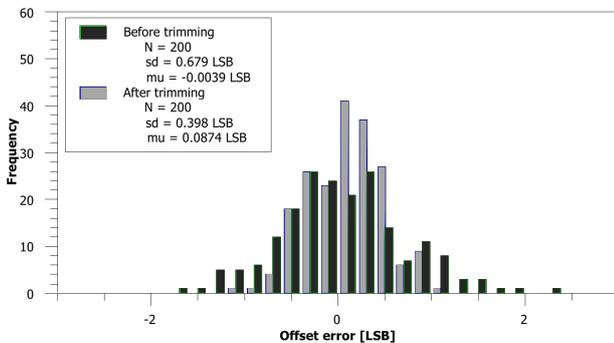
Fig. 9. Deviation of the offset error.
