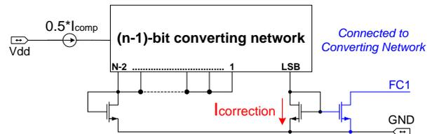
Fig. 6. Correction circuit generating the correction current.
