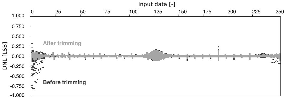
Fig. 8. Deviation of DNL versus the DAC input data code.
