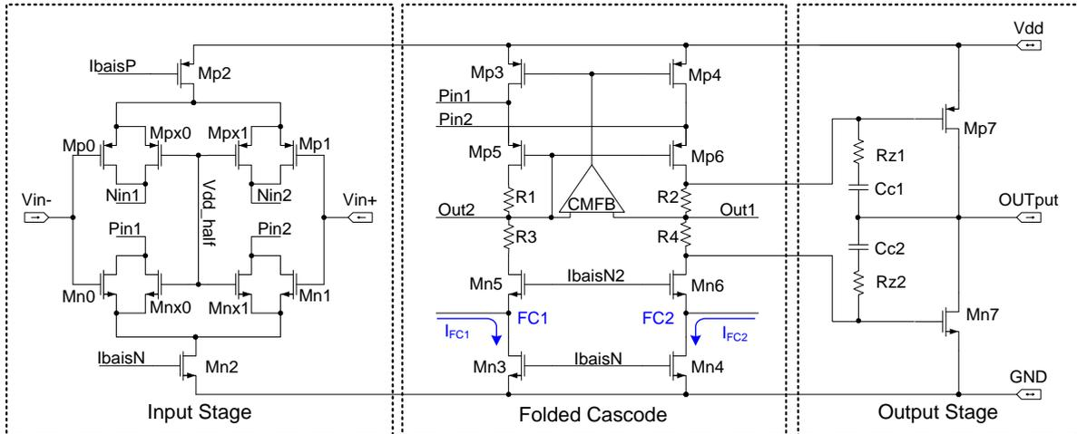
Fig. 2. Schematic diagram of the OPAMP used in DAC.
