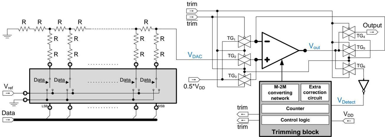
Fig. 4. Circuit diagram of the self-calibrated 8-bit R-2R DAC.
