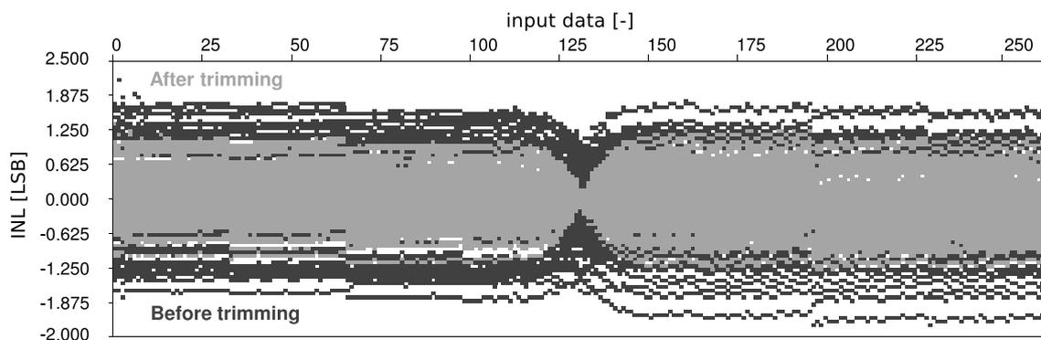
Fig. 7. Deviation of INL versus the DAC input data code.
