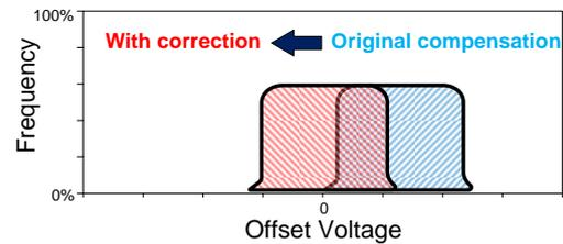
Fig. 5. Principle of the offset mean value shift by a correction circuit.
