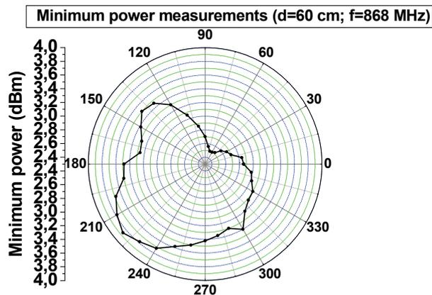
Fig. 13. Minimum power measurements vs. angle.
