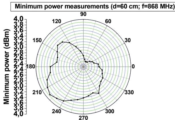
Fig. 13. Minimum power measurements vs. angle.
