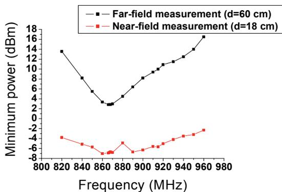
Fig. 12. Minimum power vs. frequency for near-field and far-field reading measurements.
