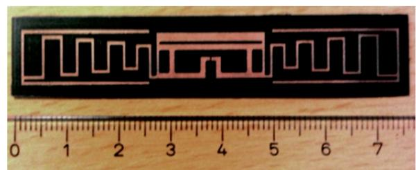
Fig. 9. UHF RFID tag used in measurements.
