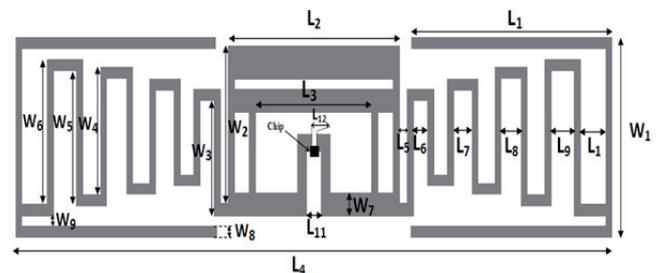
Fig. 1. Geometry of the proposed meandered antenna.
