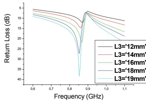
Fig. 4. Return loss of the tag antenna for various  $L_3$ .
