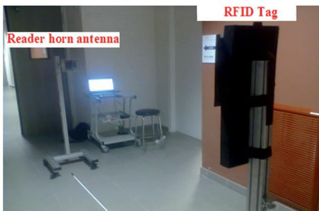
Fig. 14. Experimental setup for testing the proposed UHF RFID tag.
