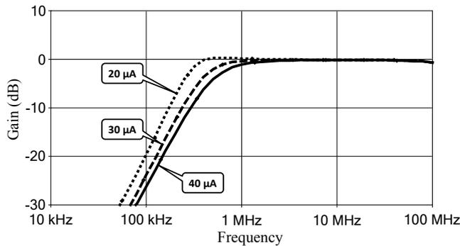
Fig. 12. Frequency responses of the filter.
