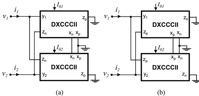
Fig. 18. DXCCCII based floating resistors a) positive resistor, b) negative resistor.
