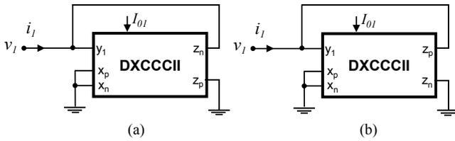
Fig. 17. DXCCCII based grounded resistors a) positive resistor, b) negative resistor.
