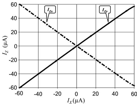
Fig. 6. The current transfer curve for the DXCCCII.
