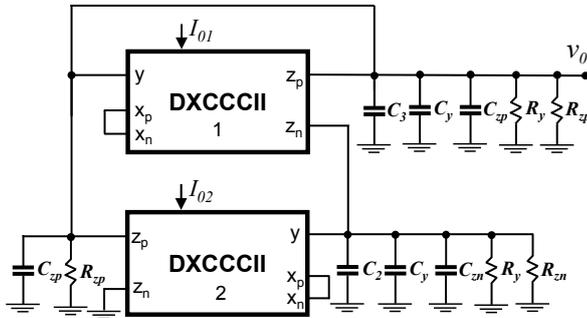
Fig. 16. The non-ideal model of the oscillator.
