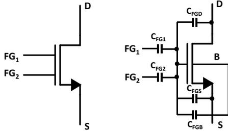
Fig. 1. The n-type FGMOS transistor with three inputs: a) symbol, b) equivalent circuit.
