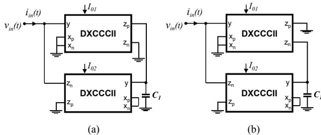
Fig. 9. Inductance simulators realized using DXCCCII: a) positive, b) negative.
