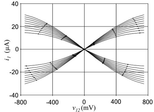
Fig. 19. The I-V characteristics of the floating positive and negative active resistor.
