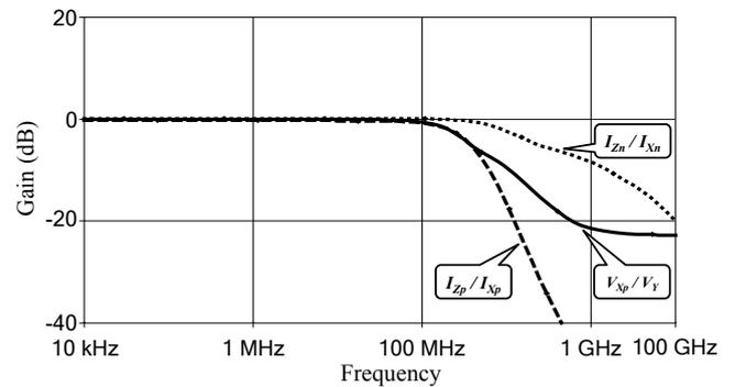
Fig. 8. The frequency response of the voltage transfer gains and current transfer gains of the proposed DXCCCII.
