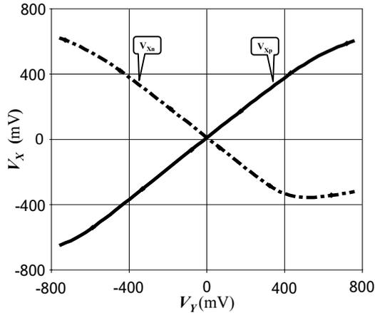
Fig. 5. The voltage transfer curve for the DXCCCII.
