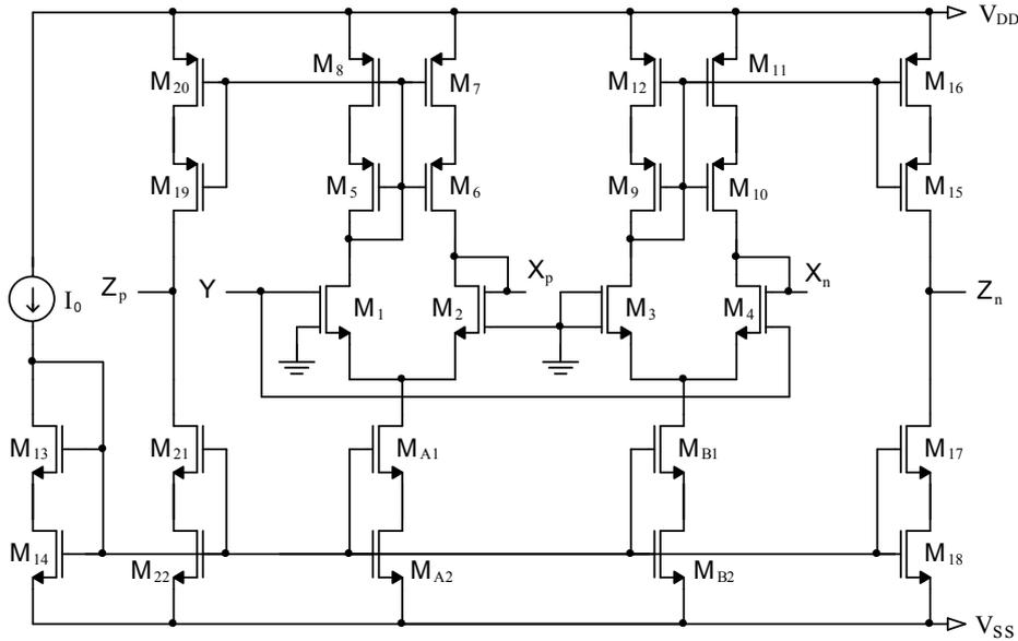
Fig. 3. The circuit structure of the DXCCCII.
