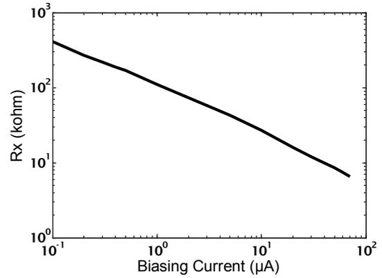
Fig. 7. The parasitic resistance of the proposed DXCCCII for different biasing currents.
