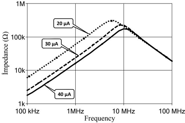
Fig. 10. The impedance values of the simulators for different biasing currents.
