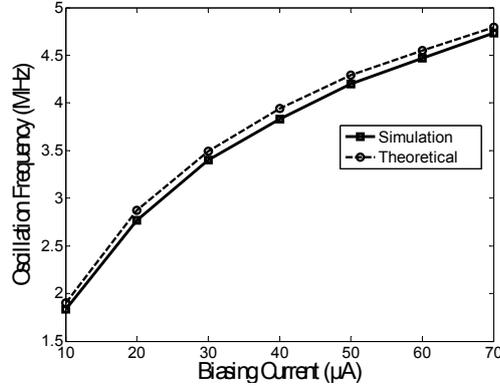
Fig. 15. Oscillation frequency versus biasing current of the second DXCCCII.
