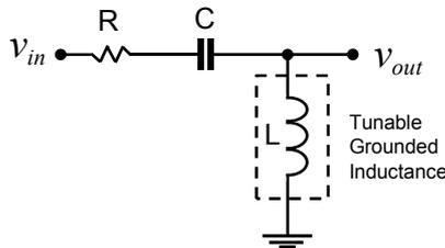
Fig. 11. The classical high pass filter.
