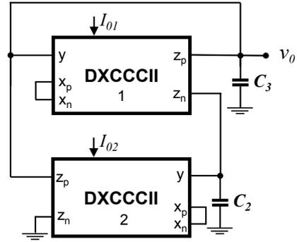
Fig. 13. The tunable oscillator circuit.
