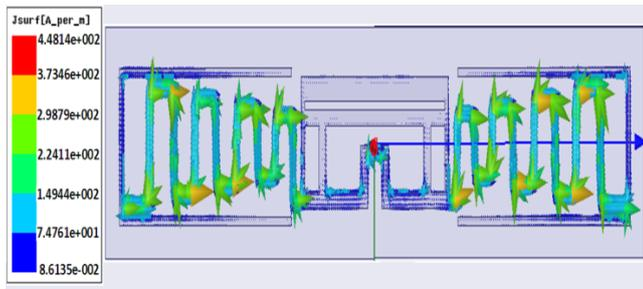
Fig. 6. Surface current distribution at 867 MHz
