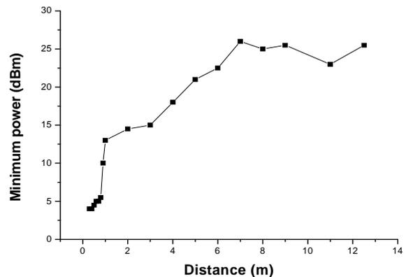
Fig. 15 Minimum power vs. distance in RFID system
