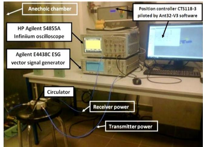
Fig. 8. Photograph of the measurement equipment
