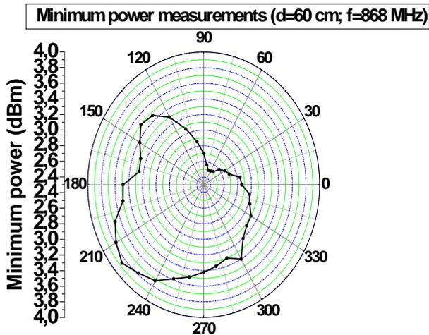
Fig. 13. Minimum power measurements vs. angle
