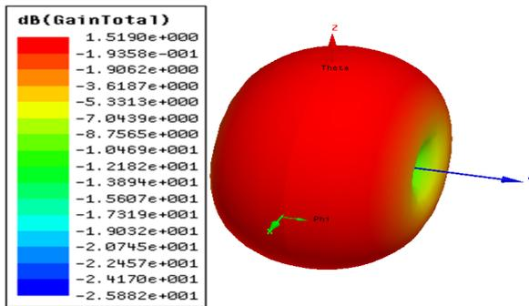
Fig. 3. 3-D far-field radiation plot at 867.7 MHz
