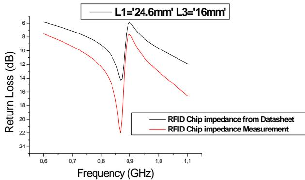
Fig. 2. Simulated return loss for the proposed broadband Tag antenna
