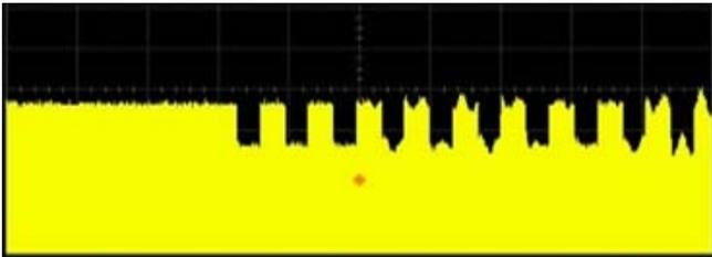
Fig. 11. Portion of the received Tag response at 867 MHz
