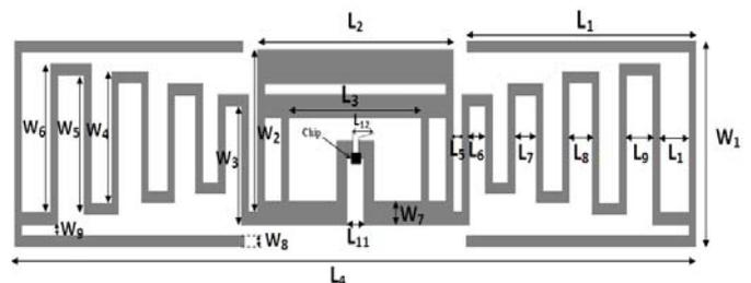
Fig. 1. Geometry of the proposed meandered antenna
