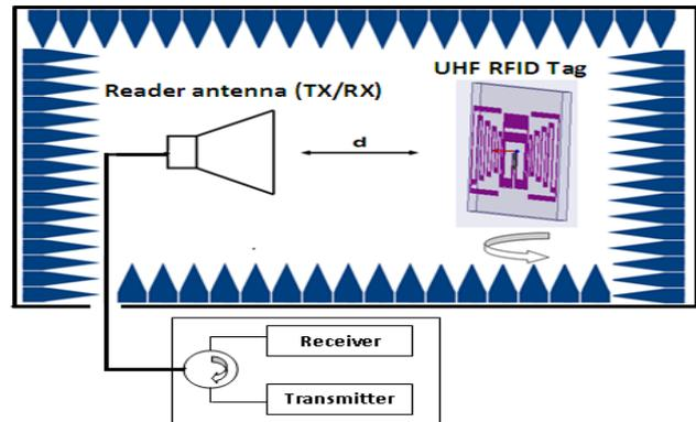
Fig. 7. Experimental setup of the Tag in the mono-static configuration
