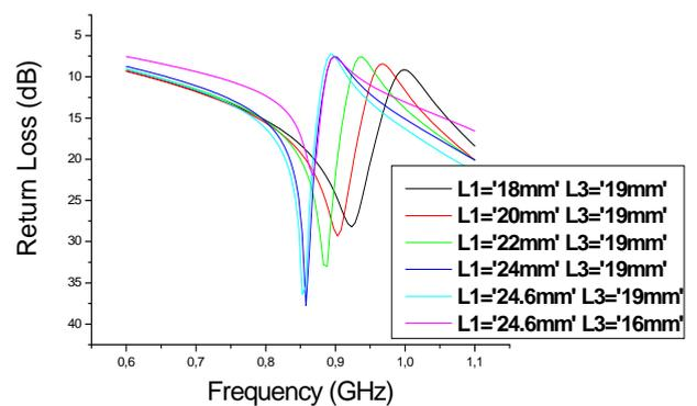
Fig. 5. Return Loss of the antenna for various  $L_1$
