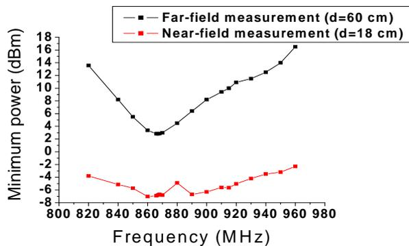
Fig. 12. Minimum power vs. frequency for near-field and far-field reading measurements
