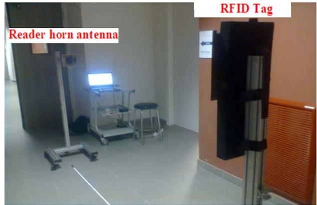
Fig. 14 Experimental setup for testing the proposed UHF RFID Tag
