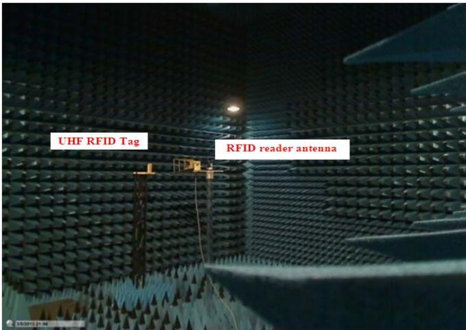
Fig. 10. UHF RFID Tag range measurement using anechoic chamber
