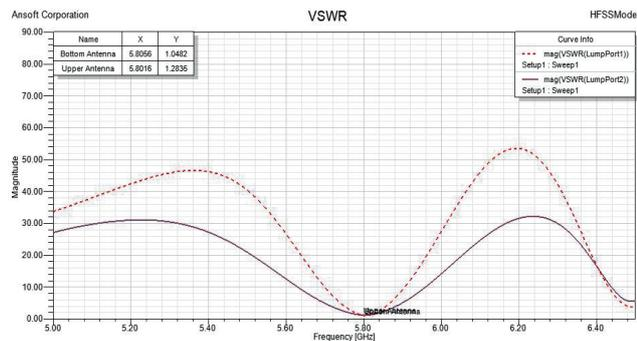
Fig. 7. VSWR plots versus frequency for SCP antenna.
