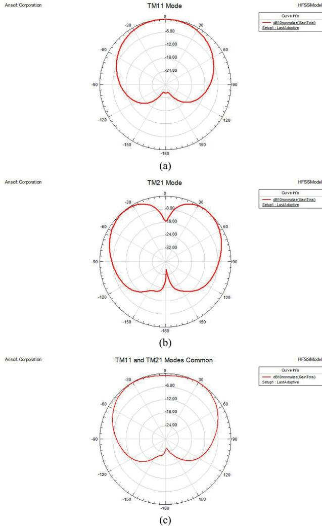
Fig. 6. Radiation patterns of SCP antenna: (a) TM11 alone, (b) TM21 alone, (c) TM11 and TM21 superimposed.
