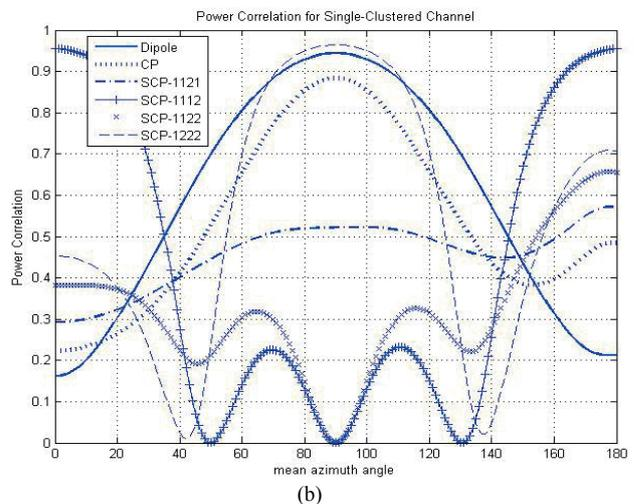
**Fig. 9.** Power correlation values of DP-ULA, CP-ULA and SCP-ULA versus mean azimuth angle (a):  $\sigma_c^2 = 5^\circ$ , (b)  $\sigma_c^2 = 20^\circ$ .
