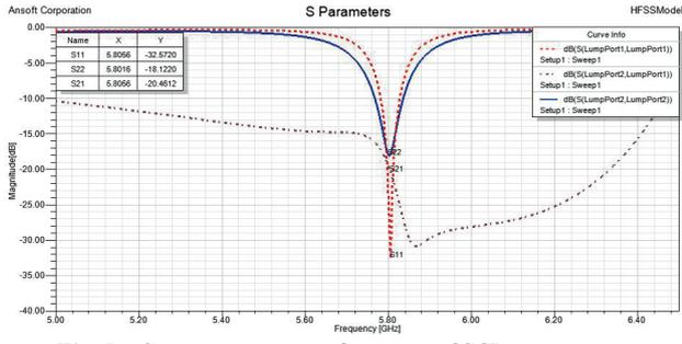
Fig. 5. S-parameters versus frequency of SCP antenna.
