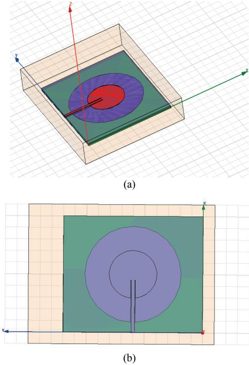
Fig. 4. The side (a) and the top (b) view of the SCP antenna with microstrip feed lines in HFSS.
