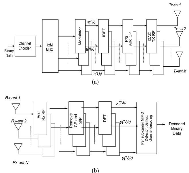
Fig. 1. Transmitter and receiver diagrams of a MIMO-OFDM WLAN system: (a) Transmitter. (b) Receiver.
