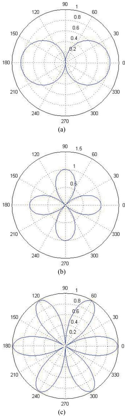
Fig. 3. Radiation patterns of multimode circular patch antennas: (a) TM11 mode, (b)TM21 mode, (c)TM31 mode.
