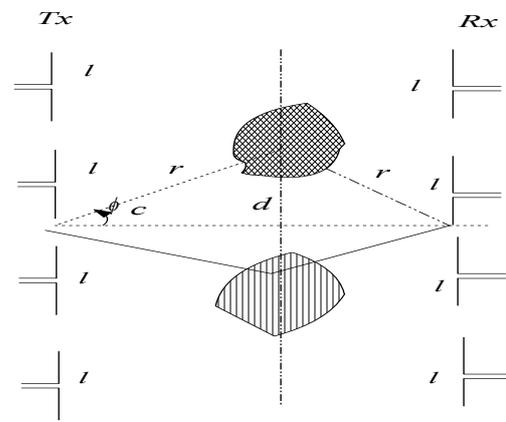
Fig. 2. Geometry of the clustered channel model representing clusters and transmit/receive antenna arrays (4x4 array) where  $\phi_0$  is the mean A.O.D. of the cluster.
