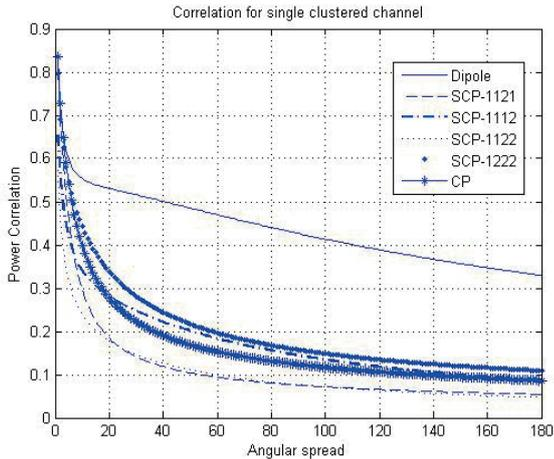
**Fig. 8.** Power correlation values of DP-ULA, CP-ULA and SCP-ULA averaged over azimuth angle  $\phi$  for a  $2 \times 2$  array.
