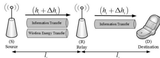
Fig. 1. The system model consists of a source, a relay and a destination node which are denoted by ( $S$ ), ( $R$ ) and ( $D$ ), respectively.
