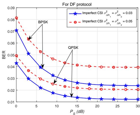
Fig. 5. BER of the AF and DF relaying networks with various values of  $P_S$ .
