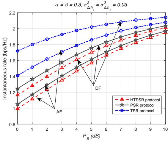
Fig. 4. The instantaneous rate of perfect and imperfect CSI for AF and DF relaying networks for different values of  $P_S$ .
