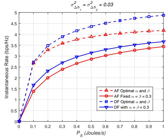
Fig. 6. Impact of optimal time switching and power splitting fraction.
