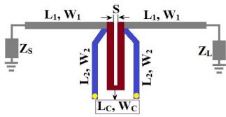
Fig. 6. The physical layout of the proposed DFIT.
