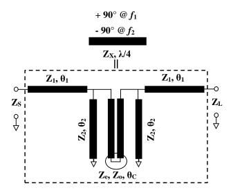
Fig. 1. Schematic of the proposed dual-frequency impedance transformer.
