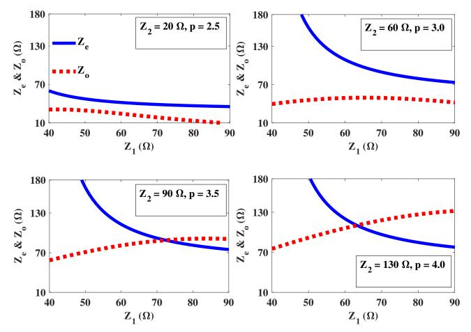
Fig. 4. The variation of even and odd-mode impedances of the coupled-line as a function of  $Z_1$  with different values of  $Z_2$  and p for a load impedance of 1000  $\Omega$ .
