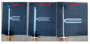
Fig. 7. Photograph of the fabricated prototypes with transforming ratios of 10, 20 and 30.
