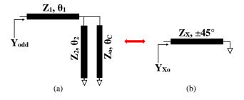
Fig. 3. Odd half-network. (a) Proposed dual-band structure. (b) Equivalent circuit.
