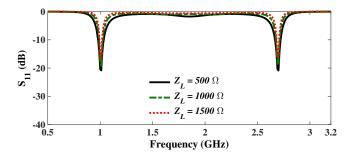
**Fig. 5.** The circuit simulated magnitude response of the DFIT with transforming ratios of 10, 20 and 30.
