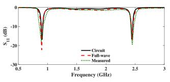
**Fig. 10.** Circuit, full-wave simulated and measured *S*<sub>11</sub> response of the UHTR-DFIT with transforming ratio of 30.
