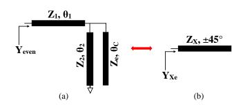
Fig. 2. Even half-network. (a) Proposed dual-band structure. (b) Equivalent circuit.
