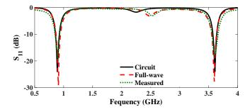
**Fig. 8.** Circuit, full-wave simulated and measured *S*<sub>11</sub> response of the UHTR-DFIT with transforming ratio of 10.
