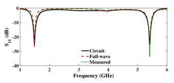
**Fig. 9.** Circuit, full-wave simulated and measured *S*<sub>11</sub> response of the UHTR-DFIT with transforming ratio of 20.
