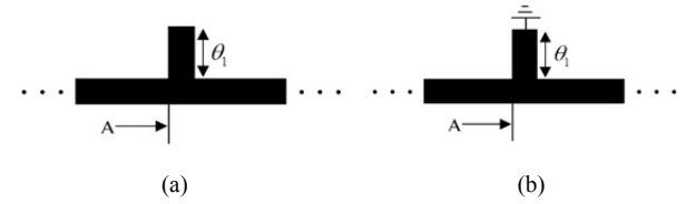
Fig. 3. Microstrip structures of Fig. 2: (a) Opened stub. (b) Shorted stub.
