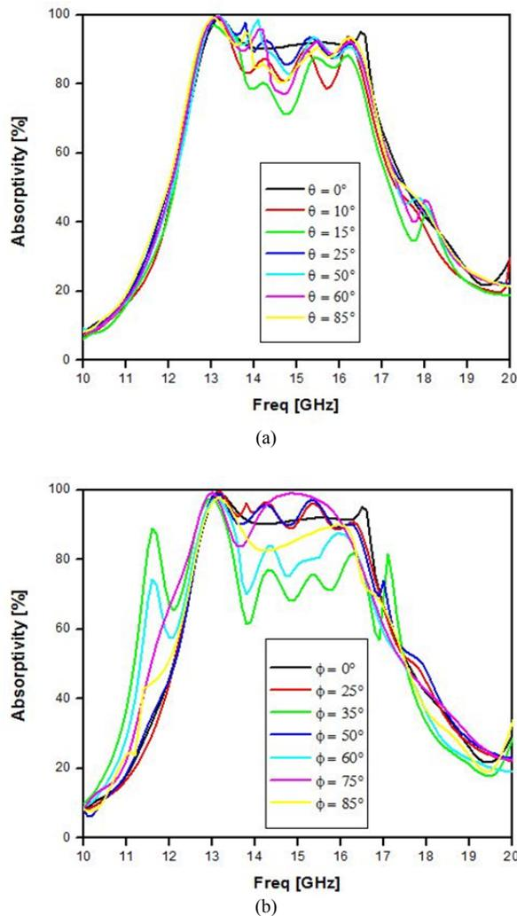
Fig. 10. Simulated absorptivities under (a) oblique and (b) normal incidence for TE polarization.
