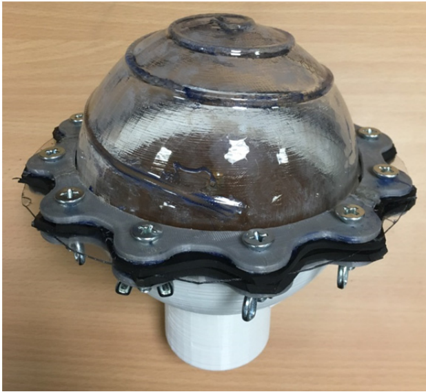
Fig. 10. Prototype of vacuum formed hemisphere with antenna glued to the small width canals on the inner surface.
