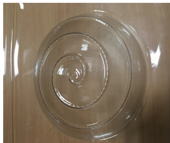
Fig. 2. Vacuumed formed hemisphere with small width canals on the inner surface.
